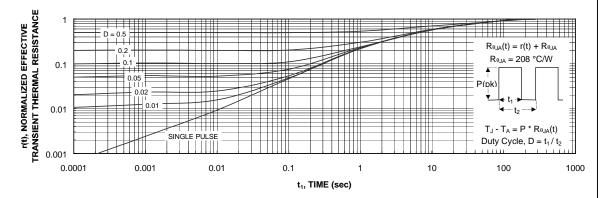
Figure 11. Transient Thermal Response Curve.
