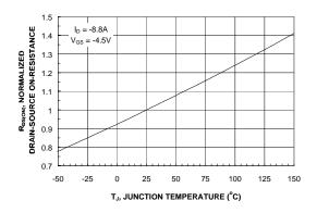
Figure 3. On-Resistance Variation with Temperature.
