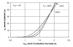
Figure 5. Transfer Characteristics.
