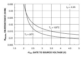
Figure 4. On-Resistance Variation with Gate-to-Source Voltage.
