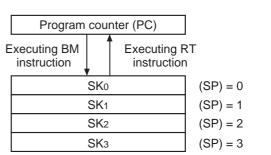
Stack pointer (SP) points "3" at reset or returning from RAM back-up mode. It points "0" by executing the first BM instruction, and the contents of program counter is stored in SKo. When the BM instruction is executed after four stack registers are used ((SP) = 3), (SP) = 0 and the contents of SKo is destroyed.
