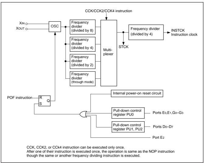
Fig. 27 Clock control circuit structure
