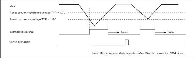
Fig. 22 Voltage drop detection circuit operation waveform
