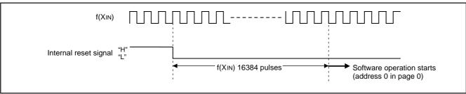
Fig. 19 Reset release timing
