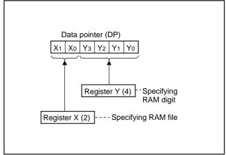
Fig. 8 Data pointer (DP) structure
