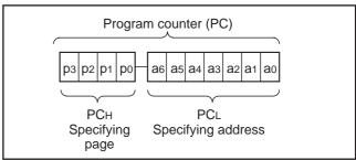
Fig. 7 Program counter (PC) structure
