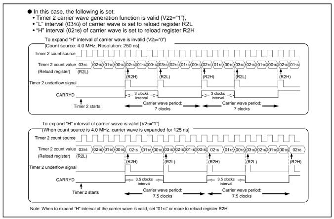
Fig. 16 Carrier wave generation example by timer 2
