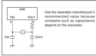
Fig. 28 Ceramic resonator external circuit
