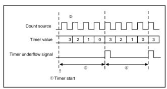
Fig. 29 Count start time and count time when operation starts (T1, T2)
