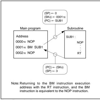
Fig. 6 Example of operation at subroutine call
