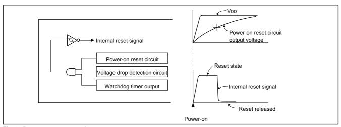
Fig. 20 Power-on reset operation
