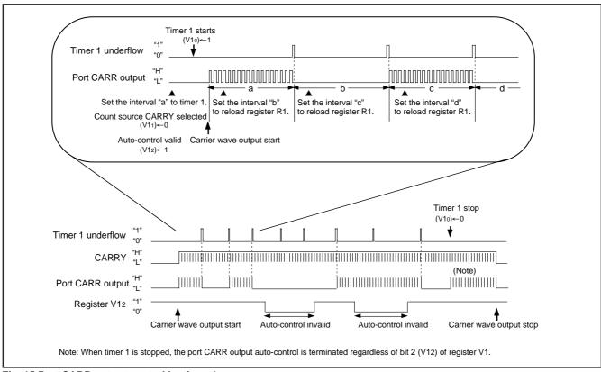
Fig. 15 Port CARR output control by timer 1
