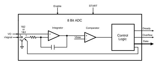
The A/D converter multiplexes 4 different sources:
