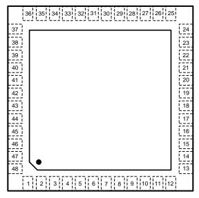
Figure 2. 48 WQFN Package (Top View) Package Number NJV0048A
