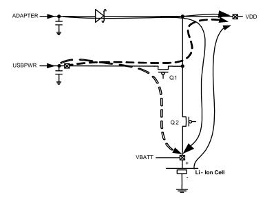
The current provided by the external adapter power or USB power, when inserted, first supplies the system load; the remainder is used for charging.
