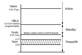
Figure 58. Voltage Threshold Levels
