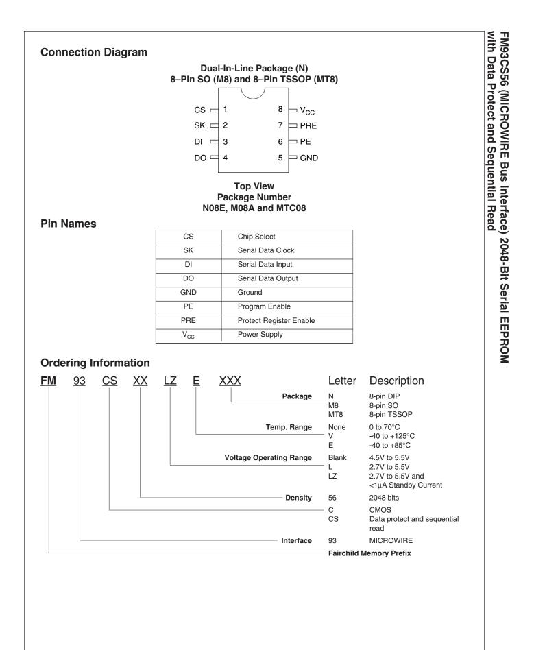
FM93CS56 (MICROWIRE Bus Interface) 2048-Bit Serial EEPROM with Data Protect and Sequential Read
