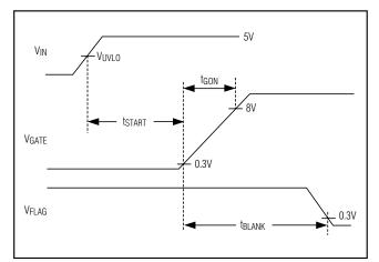
Figure 1. Startup Timing Diagram
