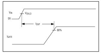
Figure 3. Power-Up Overvoltage Timing Diagram
