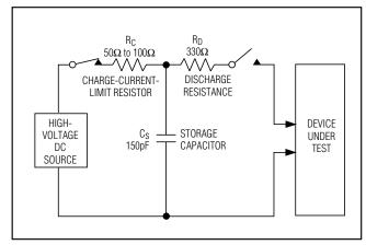
Figure 8. IEC 1000-4-2 ESD Test Model
