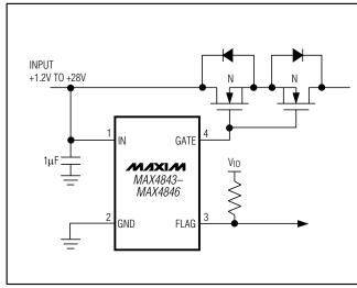
Figure 5. Back-to-Back External MOSFET Configuration
