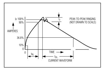
Figure 7. Human Body Model Current Waveform
