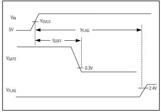
Figure 2. Shutdown Timing Diagram
