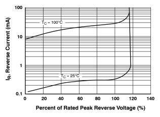
Figure 3. Reverse Current vs. Reverse Voltage
