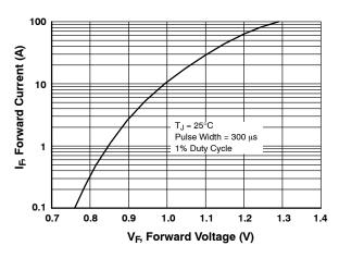
Figure 2. Forward Voltage Characteristics
