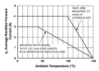
Figure 1. Forward Current Derating Curve
