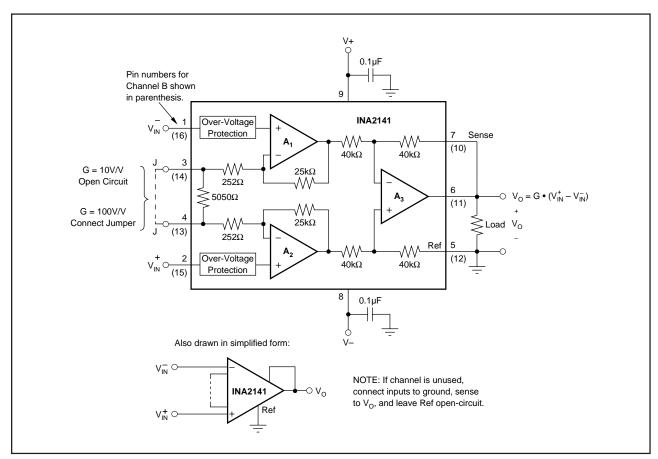
FIGURE 1. Basic Connections.
