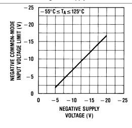
Figure 5. Negative Common-Mode Input Voltage Limit
