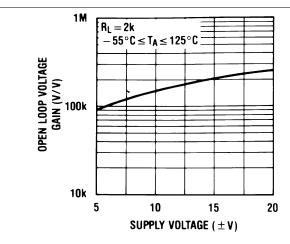
Figure 19. Open Loop Voltage Gain
