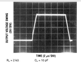
Figure 24. Large Signal Inverting
