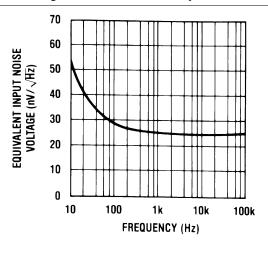
Figure 18. Equivalent Input Noise Voltage
