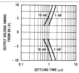
Figure 21. Inverter Settling Time
