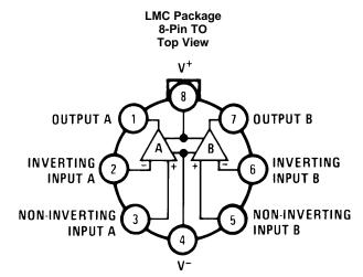
Note. Pin 4 connected to case.
