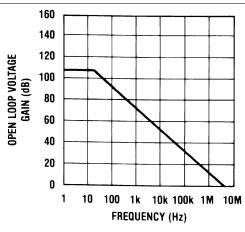
Figure 15. Open Loop Frequency Response
