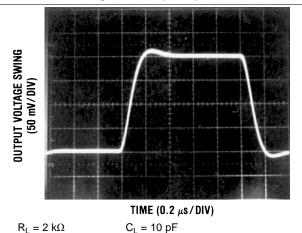
Figure 22. Small Signal Inverting
