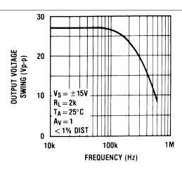
Figure 14. Undistorted Output Voltage Swing
