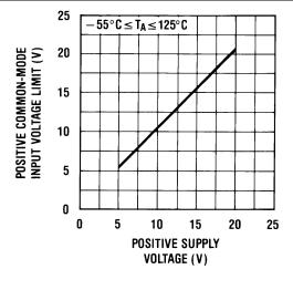
Figure 4. Positive Common-Mode Input Voltage Limit
