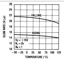
Figure 11. Bode Plot Figure 12. Slew Rate
