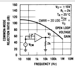
Figure 16. Common-Mode Rejection Ratio
