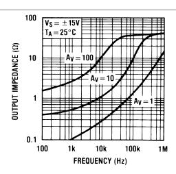
Figure 20. Output Impedance
