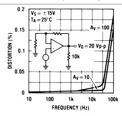
Figure 13. Distortion vs Frequency
