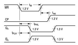
Figure 2. Master Reset to Output Delay, Master Reset Pulse Width, and Master Reset Recovery Time
