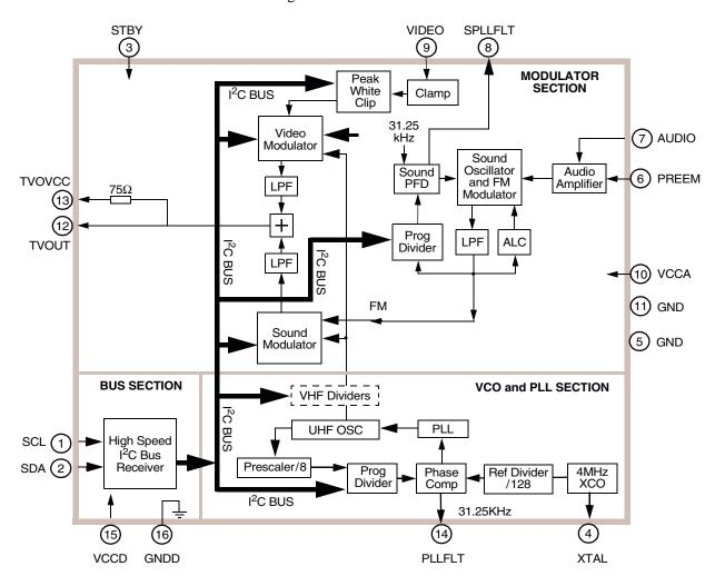
Figure 2. MC44BC374T1 Simplified Block Diagram
