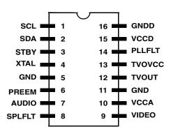
Figure 1. Pin Connection Diagram
