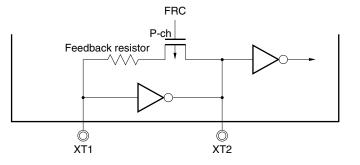
★ Remark The feedback resistor is required to control the bias point of the oscillation waveform so that the bias point is in the middle of the power supply voltage.
