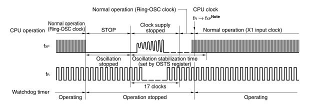
**Note** Confirm the oscillation stabilization time of fxP using the oscillation stabilization time counter status register (OSTC).
