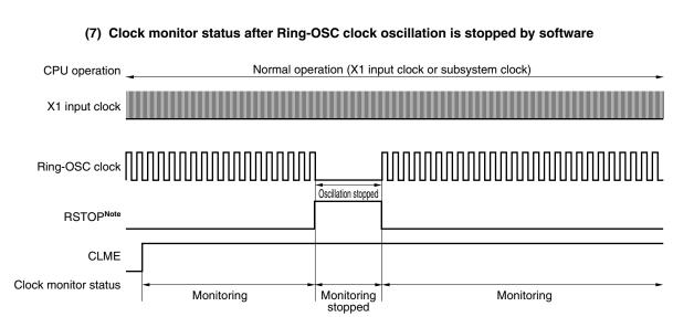
Figure 20-3. Timing of Clock Monitor (4/4)
