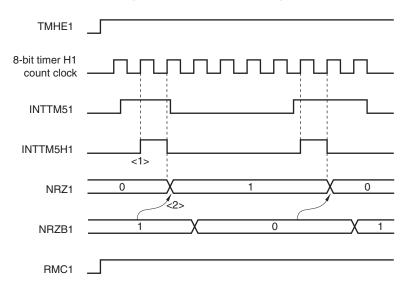
Figure 8-13. Transfer Timing
