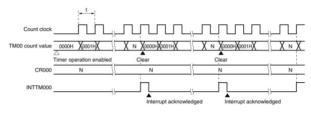
**Remark** Interval time =  $(N + 1) \times t$ N = 0001H to FFFFH
