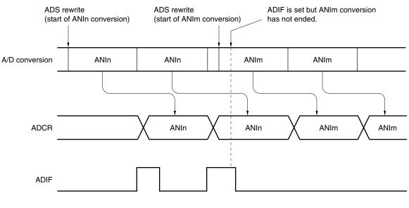
Figure 12-20. Timing of A/D Conversion End Interrupt Request Generation
