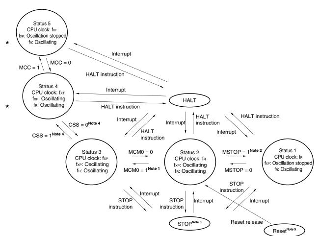
(4) When "Ring-OSC cannot be stopped" is selected by mask option (when subsystem clock is used)
