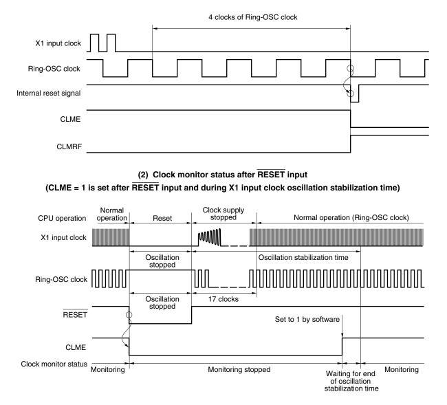
RESET input clears bit 0 (CLME) of the clock monitor mode register (CLM) to 0 and stops the clock monitor operation. Even if CLME is set to 1 by software during the oscillation stabilization time (reset value of OSTS register is 05H (2<sup>16</sup>/fxp)) of the X1 input clock, monitoring is not performed until the oscillation stabilization time of the X1 input clock ends. Monitoring is automatically started at the end of the oscillation stabilization time.
