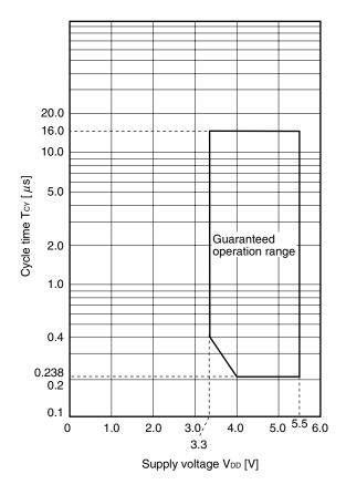
TCY vs. VDD (X1 Input Clock Operation)
