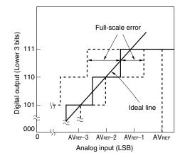
Figure 12-17. Differential Linearity Error
