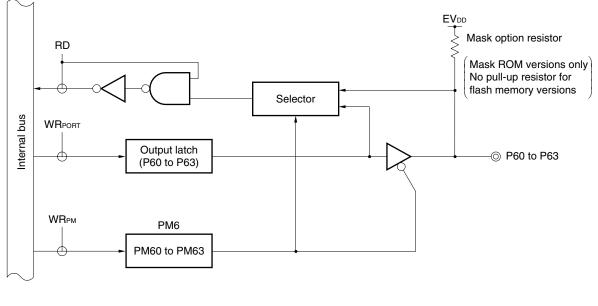
PM6:Port mode register 6RD:Read signalWRxx:Write signal
