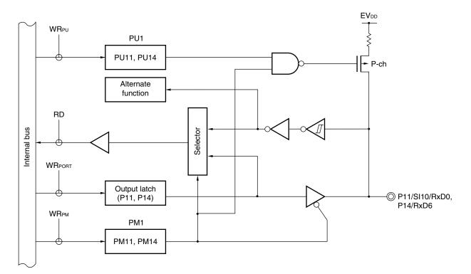
Figure 4-6. Block Diagram of P11 and P14
