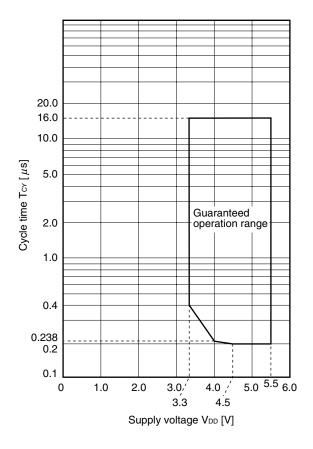
TCY vs. VDD (X1 Input Clock Operation)
