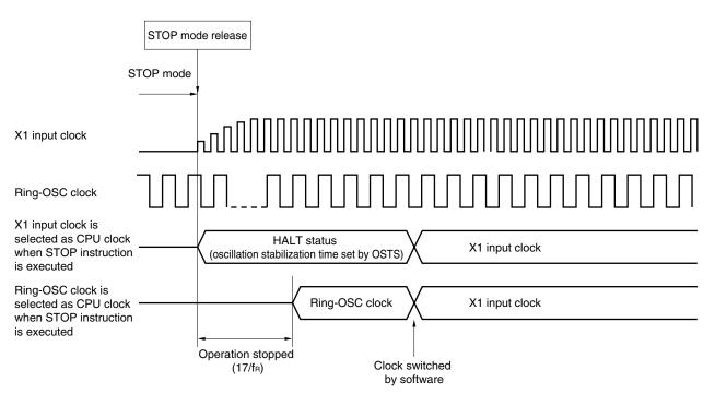
Figure 18-5. Operation Timing When STOP Mode Is Released
