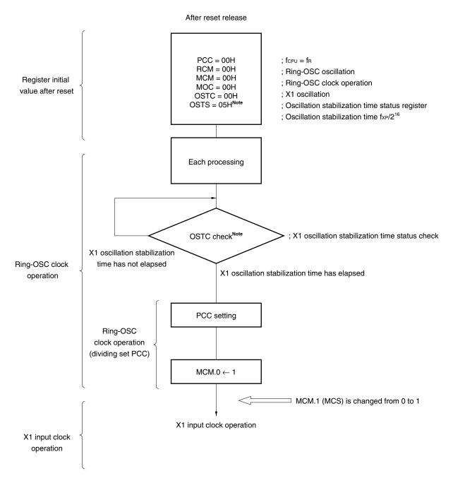
**Note** Check the oscillation stabilization wait time of the X1 oscillator after reset release using the OSTC register and then switch to the X1 input clock operation after the oscillation stabilization wait time has elapsed. The OSTS register setting is valid only after STOP mode is released by interrupt during X1 input clock operation.
