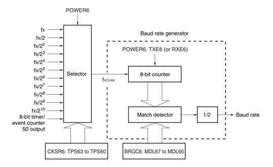
Figure 14-25. Configuration of Baud Rate Generator
