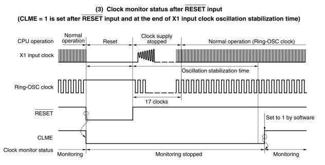
RESET input clears bit 0 (CLME) of the clock monitor mode register (CLM) to 0 and stops the clock monitor ★ operation. When CLME is set to 1 by software at the end of the oscillation stabilization time (reset value of OSTS register is 05H (2<sup>16</sup>/fx<sub>P</sub>)) of the X1 input clock, monitoring is started.
