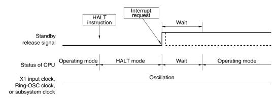
**Remarks 1.** The broken lines indicate the case when the interrupt request which has released the standby mode is acknowledged.
