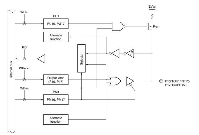
Figure 4-9. Block Diagram of P16 and P17
