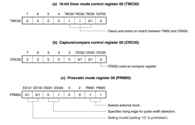
**Remark** 0/1: Setting 0 or 1 allows another function to be used simultaneously with the external event counter. See the description of the respective control registers for details.
