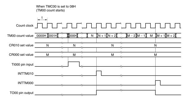
Caution 16-bit timer counter 00 starts operating as soon as a value other than 00 (operation stop mode) is set to the TMC002 and TMC003 bits.
