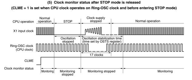
When bit 0 (CLME) of the clock monitor mode register (CLM) is set to 1 before entering STOP mode, monitoring automatically starts at the end of the X1 input clock oscillation stabilization time. Monitoring is stopped in STOP mode and during the oscillation stabilization time.
