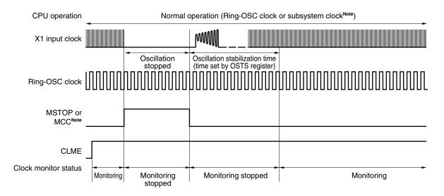
When bit 0 (CLME) of the clock monitor mode register (CLM) is set to 1 before or while oscillation of the X1 input clock is stopped, monitoring automatically starts at the end of the X1 input clock oscillation stabilization time. Monitoring is stopped when oscillation of the X1 input clock is stopped and during the oscillation stabilization time.
