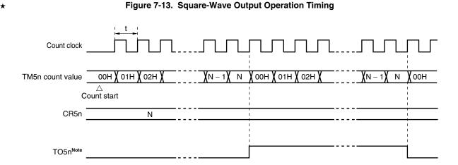
**Note** The initial value of TO5n output can be set by bits 2 and 3 (LVR5n, LVS5n) of 8-bit timer mode control register 5n (TMC5n).
