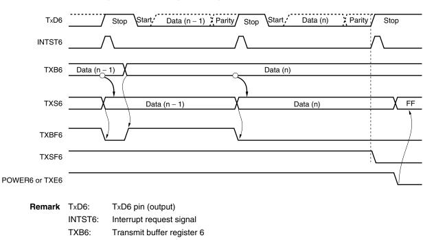
Asynchronous serial interface transmission status register 6
