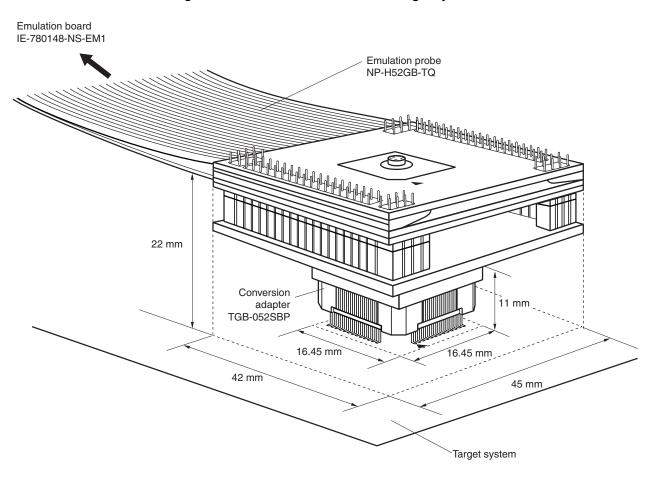
Figure B-2. Connection Conditions of Target System
