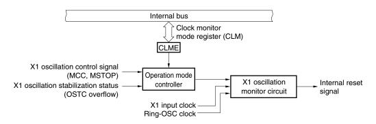
**Remark** MCC: Bit 7 of the processor clock control register (PCC)
