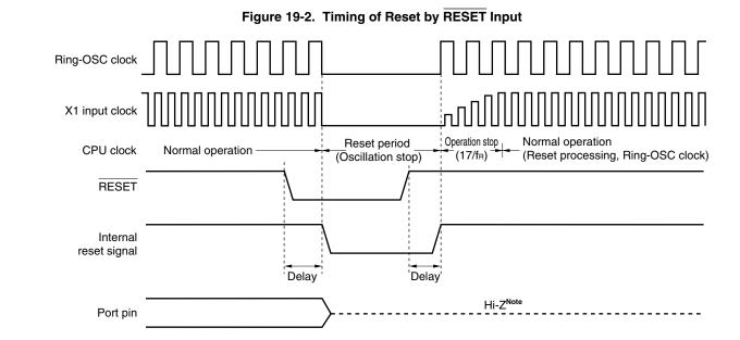
Note The port pins become high impedance, except for P130, which is set to low-level output.
