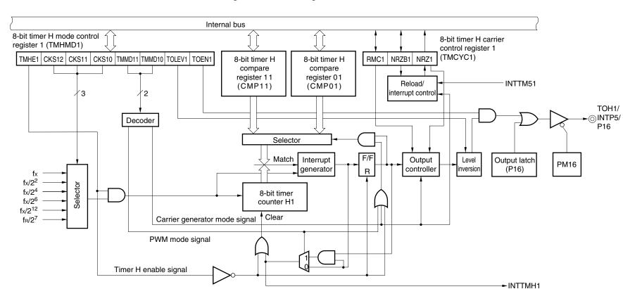
\* Figure 8-2. Block Diagram of 8-Bit Timer H1
