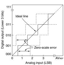
Figure 12-14. Zero-Scale Error
