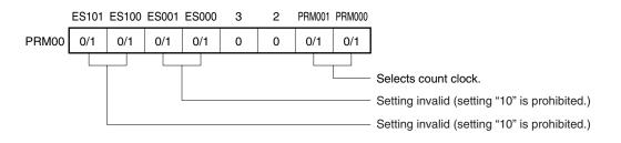
**Remark** 0/1: Setting 0 or 1 allows another function to be used simultaneously with square-wave output. See the description of the respective control registers for details.
