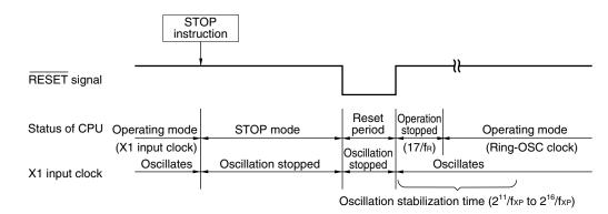
(2) When Ring-OSC clock is used as CPU clock
