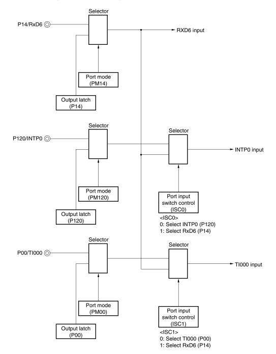
Figure 14-3. Port Configuration for LIN Reception Operation
