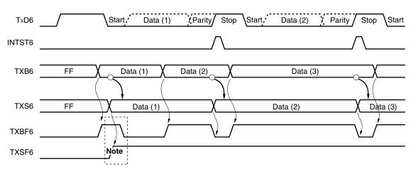
Figure 14-17. Timing of Starting Continuous Transmission
