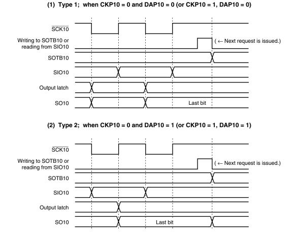
Figure 15-8. Output Value of SO10 Pin (Last Bit)
