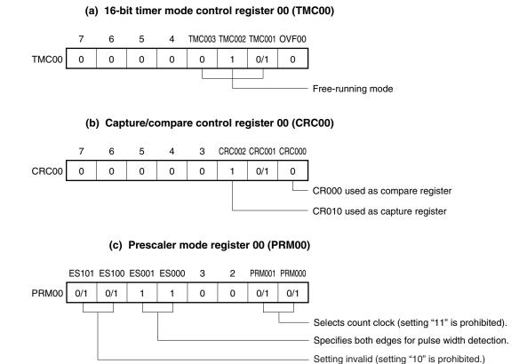
**Remark** 0/1: Setting 0 or 1 allows another function to be used simultaneously with pulse width measurement. See the description of the respective control registers for details.
