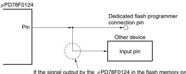
If the signal output by the  $\mu$ PD78F0124 in the flash memory programming mode affects the other device, isolate the signal of the other device.
