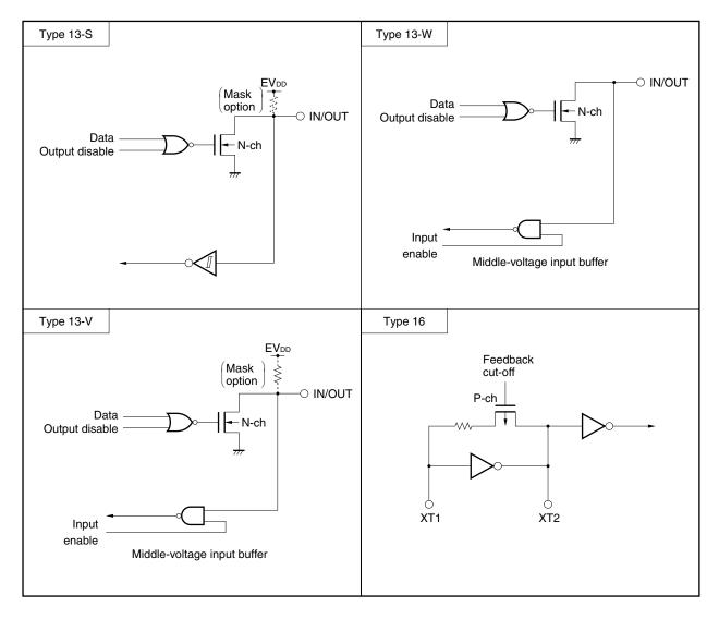
Figure 2-1. Pin I/O Circuit List (2/2)
