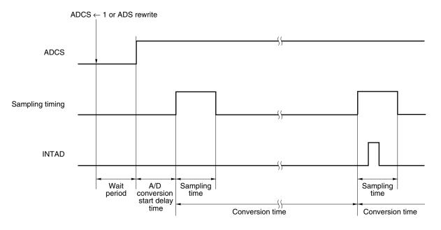
Table 12-3. A/D Converter Sampling Time and A/D Conversion Start Delay Time (ADM Set Value)
