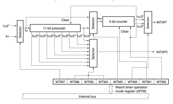
Figure 9-1. Watch Timer Block Diagram
