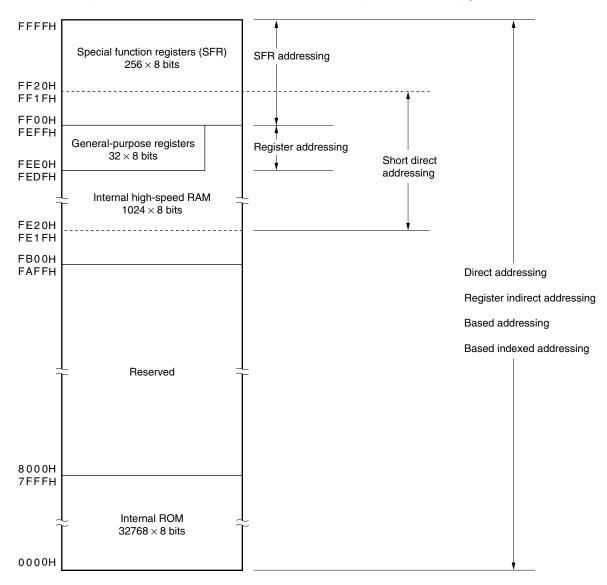
Figure 3-9. Correspondence Between Data Memory and Addressing (µPD780124)
