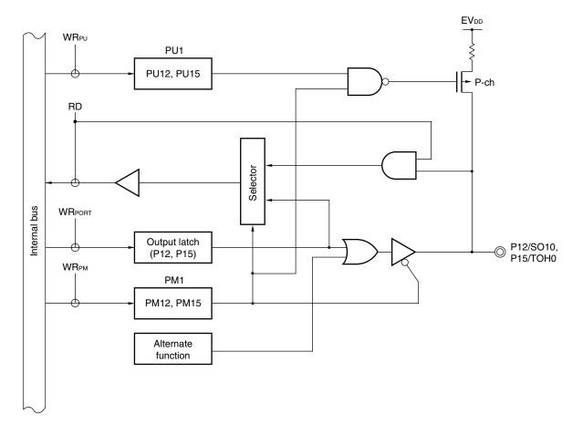
Figure 4-7. Block Diagram of P12 and P15
