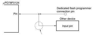
If the signal output by the dedicated flash programmer in the flash memory programming mode affects the other device, isolate the signal of the other device.
