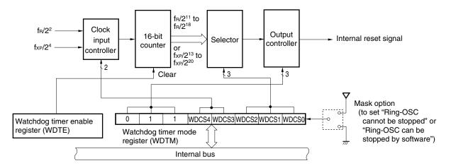
Figure 10-1. Block Diagram of Watchdog Timer
