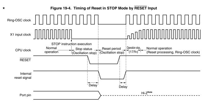
Note The port pins become high impedance, except for P130, which is set to low-level output.
