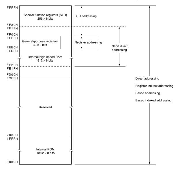
Figure 3-6. Correspondence Between Data Memory and Addressing (µPD780121)
