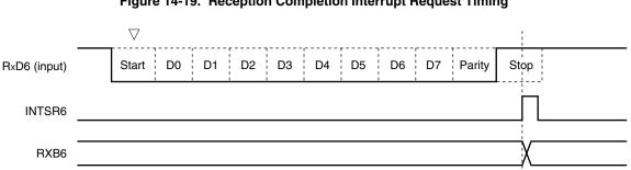
Figure 14-19. Reception Completion Interrupt Request Timing
