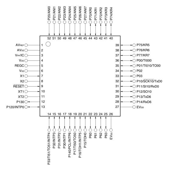
Cautions 1. Connect the IC (Internally Connected) pin directly to Vss.
