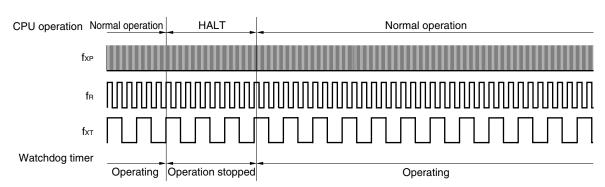
Figure 10-8. Operation in HALT Mode
