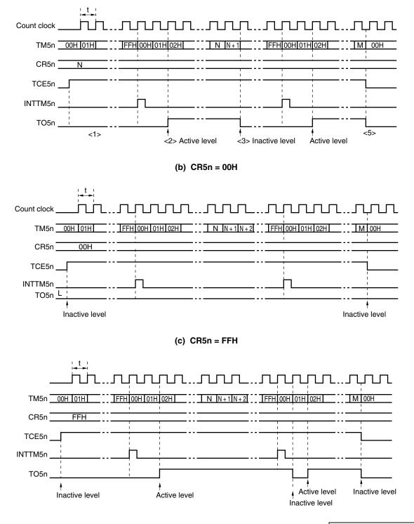
★ Remarks 1. <1> to <3> and <5> in Figure 7-14 (a) correspond to <1> to <3> and <5> in PWM output operation in 7.4.4 (1) PWM output basic operation.
