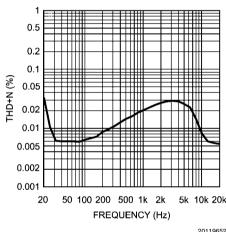
THD+N vs Frequency  $V_{DD} = 15V, R_L = 32\Omega, P_O = 20mW$
