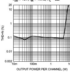
THD+N vs Output Power Per Channel  $V_{DD} = 15V$ ,  $f_{IN} = 1$ kHz,  $R_L = 8\Omega$
