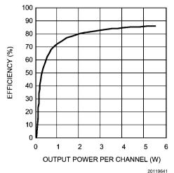
Efficiency vs Output Power  $V_{DD} = 15V, R_L = 8\Omega$
