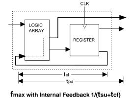
**Note:** tcf is a calculated value, derived by subtracting tsu from the period of fmax w/internal feedback (tcf = 1/fmax - tsu). The value of tcf is used primarily when calculating the delay from clocking a register to a combinatorial output (through registered feedback), as shown above. For example, the timing from clock to a combinatorial output is equal to tcf + tpd.
