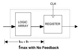
Note: fmax with no feedback may be less than 1/(twh + twl). This is to allow for a clock duty cycle of other than 50%.
