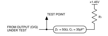
$^{*}C_{L}$  includes test fixture and probe capacitance.
