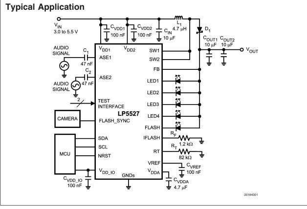
est and Audio Synchronization P5527 Tiny LED Driver for Camera Flash and 4 LEDs with I<sup>2</sup>C Programmability, Connectivity
