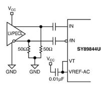
Figure 3b. LVPECL Interface (AC-Coupled)
