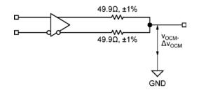
Figure 4b. LVDS Common Mode Measurement
