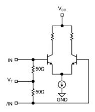
Figure 2. Simplified Differential Input Stage
