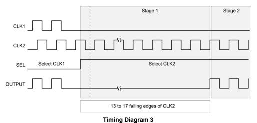
**Case #4: Input Clock Failure:** Switching from the selected clock input stuck in an undetermined state to a valid clock input (RPE enabled).
