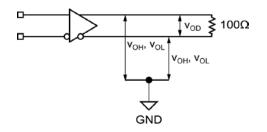
Figure 4a. LVDS Differential Measurement
