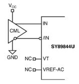
Option: may connect V<sub>T</sub> to V<sub>CC</sub> Figure 3c. CML Interface (DC-Coupled)
