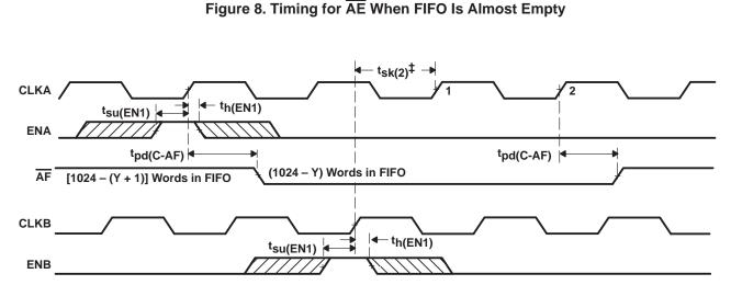
‡ t<sub>Sk(2)</sub> is the minimum time between a rising CLKA edge and a rising CLKB edge for AF to transition high in the next CLKA cycle. If the time between the rising CLKB edge and rising CLKA edge is less than t<sub>Sk(2)</sub>, AF can transition high one CLKA cycle later than shown. NOTE A: FIFO write (CSA = L, W/RA = H, MBA = L), FIFO read (CSB = L, W/RB = H, MBB = L)
