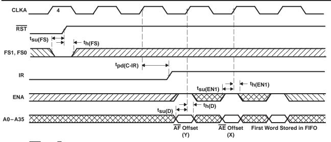
NOTE A:  $\overline{CSA} = L$ ,  $W/\overline{R}A = H$ , MBA = L. It is not necessary to program offset register on consecutive clock cycles.
