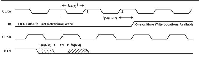
t tsk(1) is the minimum time between a rising CLKB edge and a rising CLKA edge for IR to transition high in the next CLKA cycle. If the time between the rising CLKB edge and rising CLKA edge is less than tsk(1), IR can transition high one CLKA cycle later than shown.
