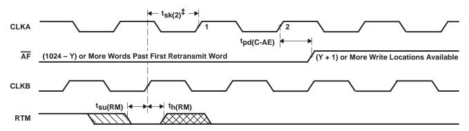
t<sub>sk(2)</sub> is the minimum time between a rising CLKB edge and a rising CLKA edge for AF to transition high in the next CLKA cycle. If the time between the rising CLKB edge and rising CLKA edge is less than t<sub>sk(2)</sub>, AF can transition high one CLKA cycle later than shown. NOTE A: Y is the value loaded in the AF flag offset register.
