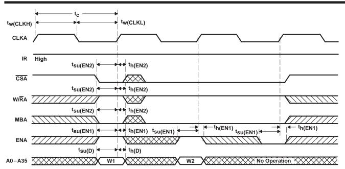
Figure 4. FIFO Write-Cycle Timing
