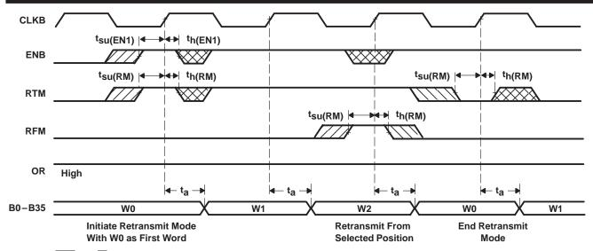
NOTE A: CSB = L, W/RB = H, MBB = L. No input enables other than RTM and RFM are needed to control retransmit mode or begin a retransmit. Other enables are shown only to relate retransmit operations to the FIFO output register.
