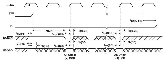
NOTE A: It is not necessary to program offset register bits on consecutive clock cycles. FIFO write attempts are ignored until IR is set high.
