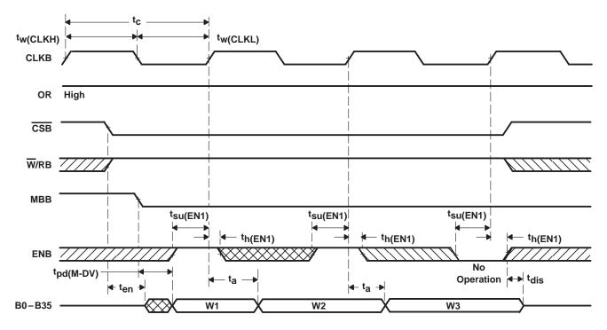
Figure 5. FIFO Read-Cycle Timing
