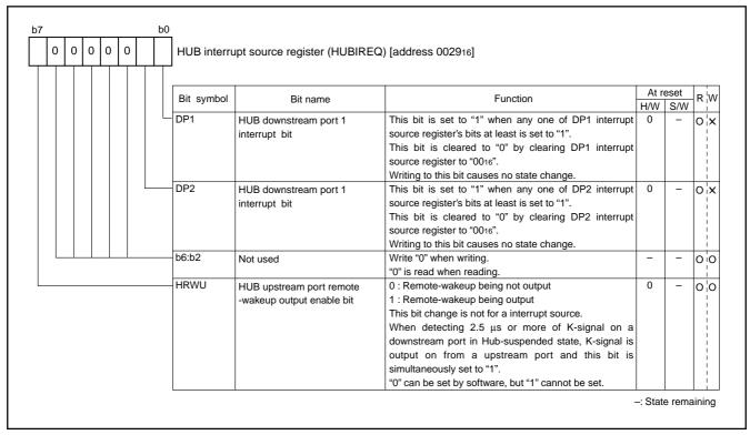
Fig. 94 Structure of HUB interrupt source register
