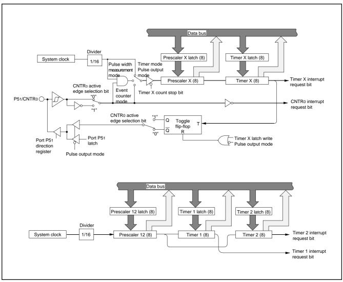
Fig. 17 Timer block diagram
