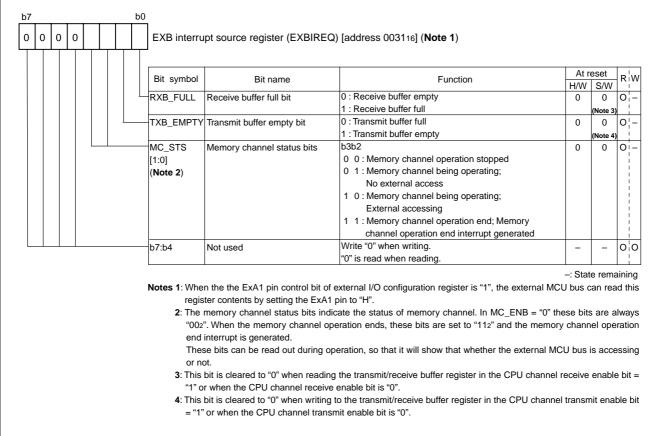
Fig. 110 Structure of EXB interrupt source register
