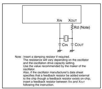
Fig. 141 Ceramic resonator or quartz-crystal oscilltor circuit
