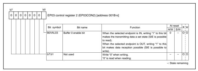
Fig. 67 Structure of EP03 control register 2
