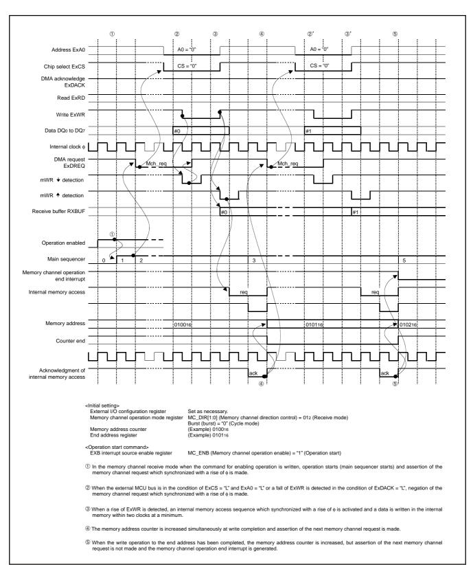
Fig. 124 Memory channel receiving operation (1)
