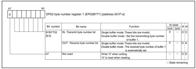
Fig. 62 Structure of EP02 byte number register 1
