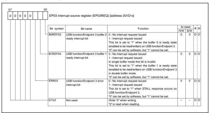
Fig. 69 Structure of EP03 interrupt source register
