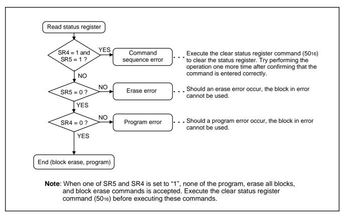
Fig. 151 Full status check flowchart and remedial procedure for errors
