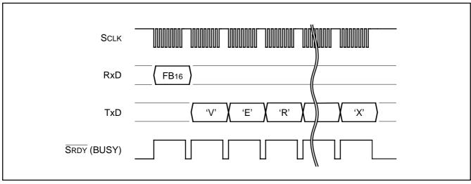
Fig. 161 Timing for version information output
