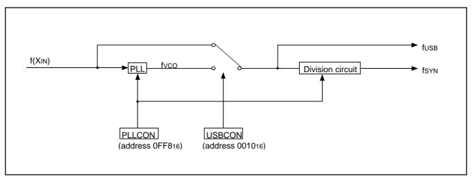
Fig. 139 Block diagram of PLL circuit
