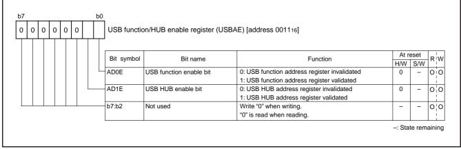
Fig. 32 Structure of USB function/HUB enable register
