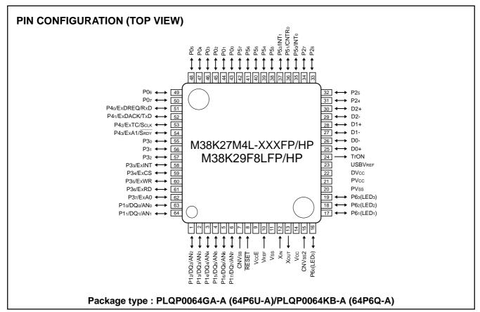
Fig. 1 Pin configuration of 38K2 group
