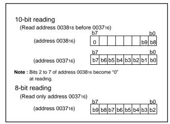
Fig. 133 10-bit/8-bit reading
