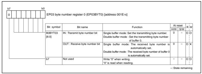
Fig. 70 Structure of EP03 byte number register 0
