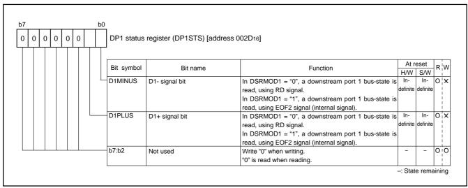
Fig. 98 Structure of DP1 status register
