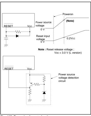
Fig. 137 Example of reset circuit
