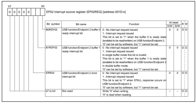
Fig. 60 Structure of EP02 interrupt source register
