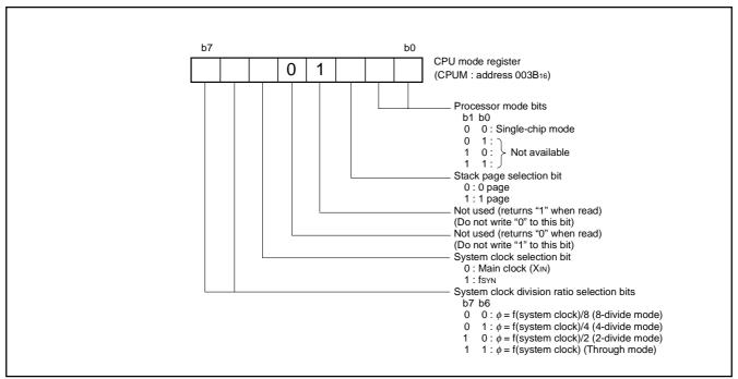
Fig. 7 Structure of CPU mode register
