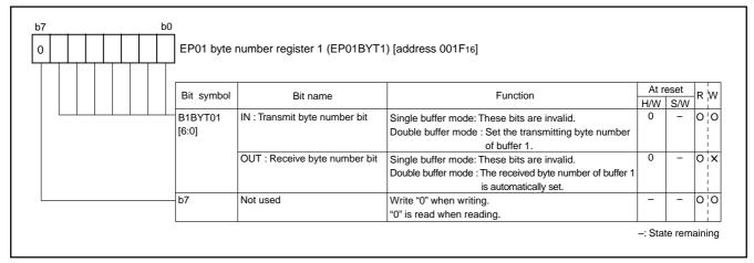
Fig. 53 Structure of EP01 byte number register 1
