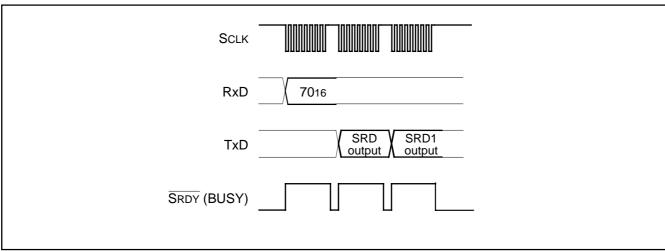
Fig. 156 Timing for reading status register
