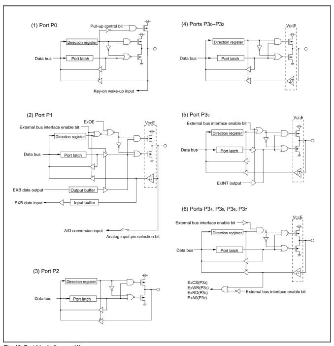
Fig. 10 Port block diagram (1)
