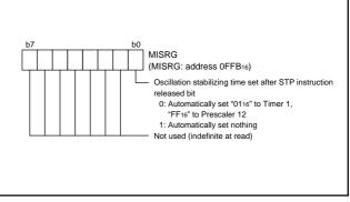
Fig. 143 Structure of MISRG
