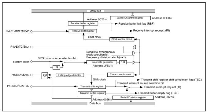
Fig. 18 Block diagram of clock synchronous serial I/O
