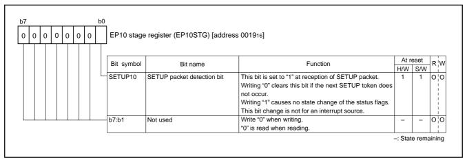
Fig. 74 Structure of EP10 stage register
