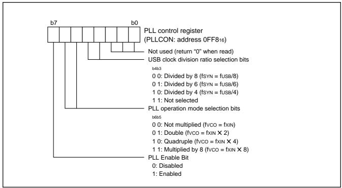
Fig. 140 Structure of PLL control register
