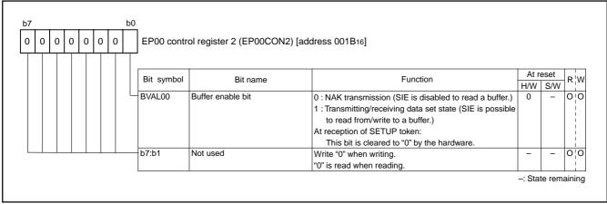
Fig. 42 Structure of EP00 control register 2
