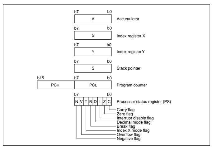
Fig. 5 740 Family CPU register structure
