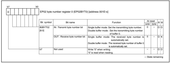
Fig. 61 Structure of EP02 byte number register 0
