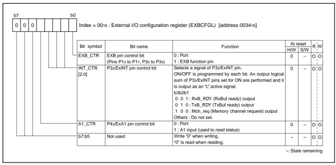
Fig. 114 Index00[low]; Structure of External I/O configuration register
