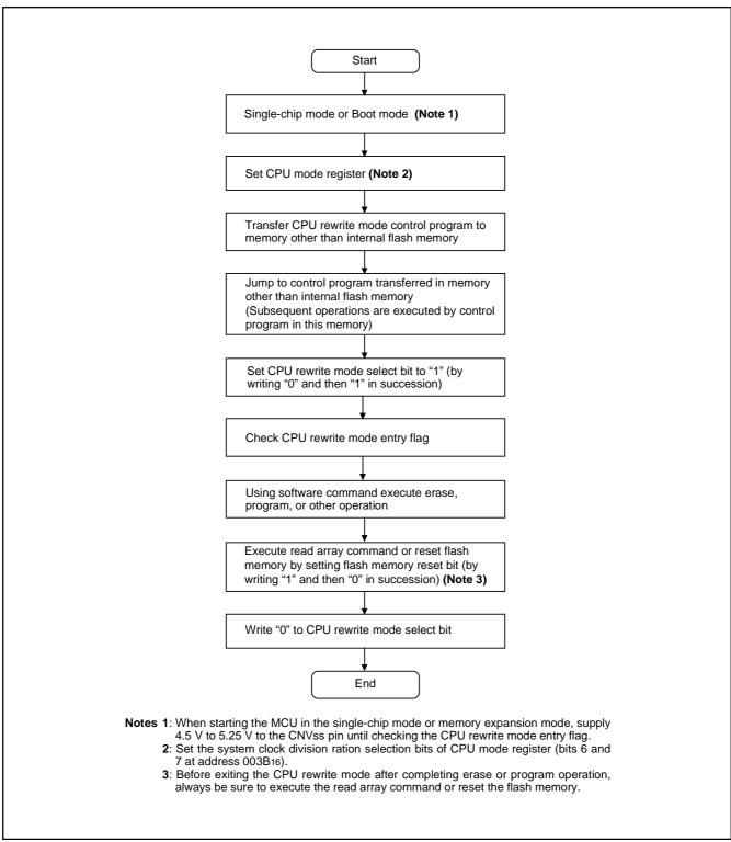
Fig. 148 CPU rewrite mode set/release flowchart
