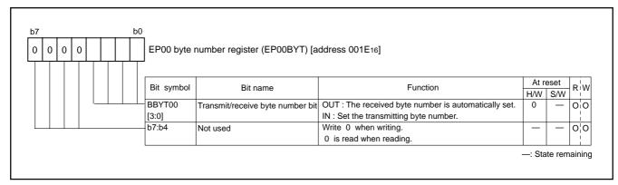
Fig. 45 Structure of EP00 byte number register
