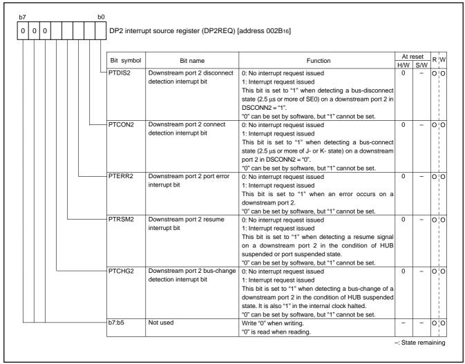
Fig. 99 Structure of DP2 interrupt source register
