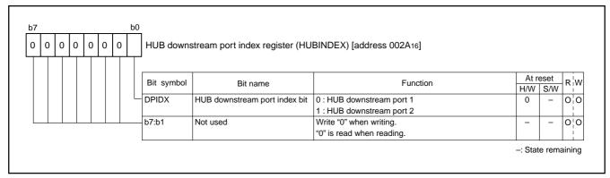
Fig. 95 Structure of HUB downstream port index register
