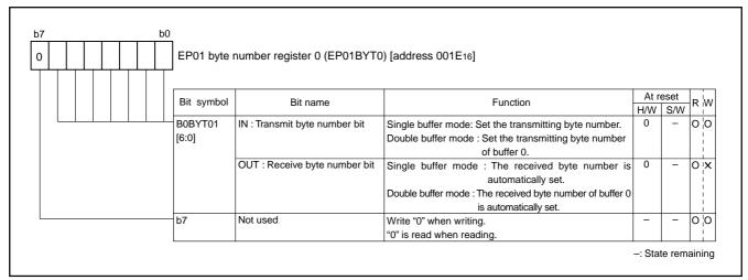
Fig. 52 Structure of EP01 byte number register 0
