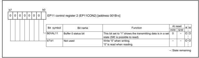
Fig. 83 Structure of EP11 control register 2
