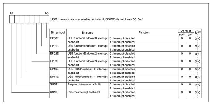
Fig. 37 Structure of USB interrupt source enable register
