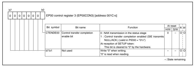
Fig. 43 Structure of EP00 control register 3
