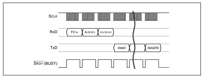
Fig. 162 Timing for Boot ROM area output
