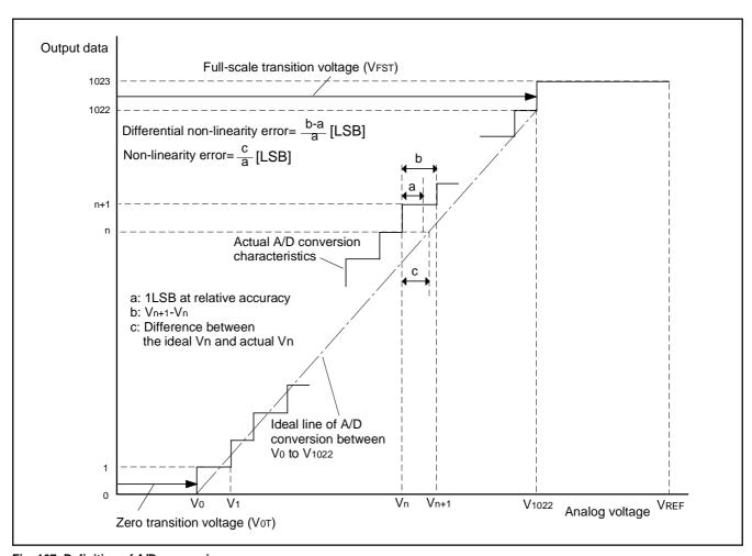
Fig. 167 Definition of A/D conversion accuracy
