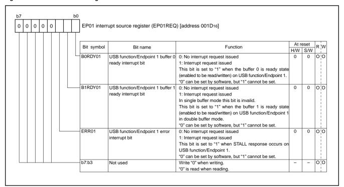
Fig. 51 Structure of EP01 interrupt source register
