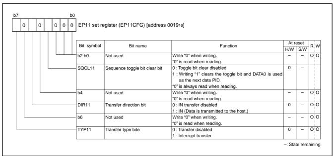
Fig. 81 Structure of EP11 set register
