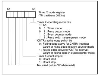
Fig. 16 Structure of timer X mode register
