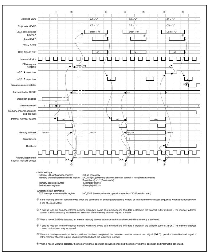
Fig. 128 Memory channel tranmitting operation (2)
