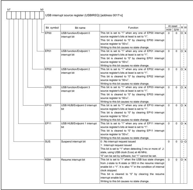
Fig.38 Structure of USB interrupt source register
