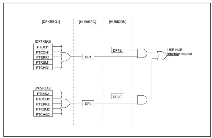
Fig. 91 USB HUB interrupt control
