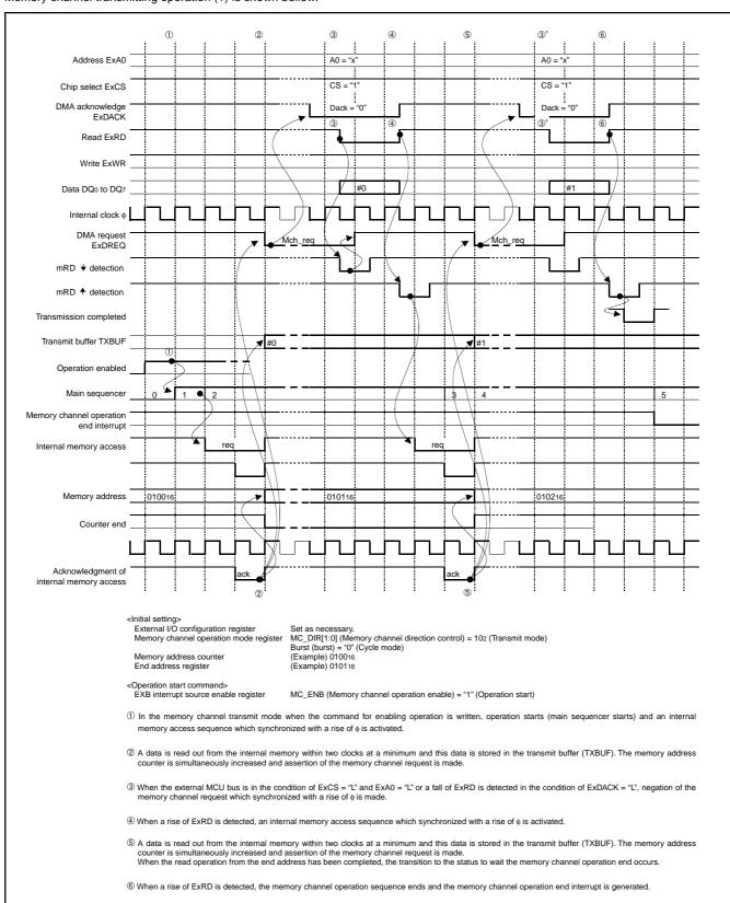
Fig. 127 Memory channel tranmitting operation (1)
