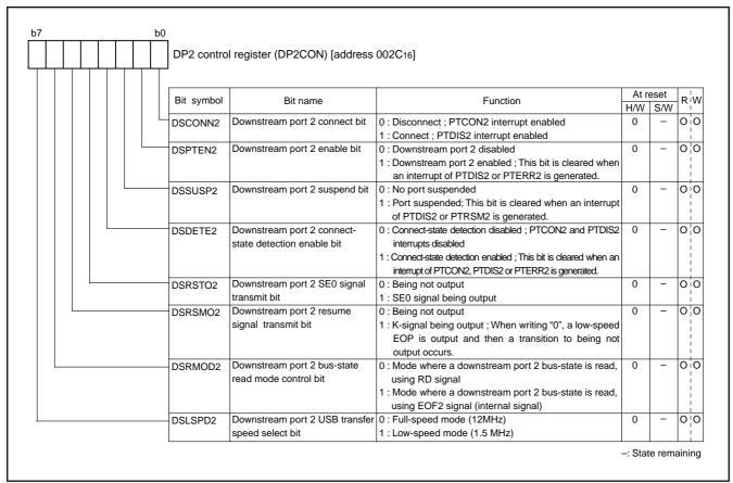
Fig. 100 Structure of DP2 control register
