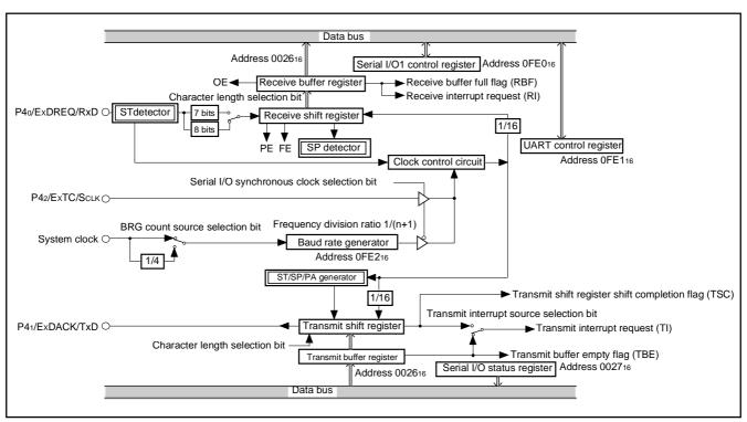
Fig. 20 Block diagram of UART serial I/O
