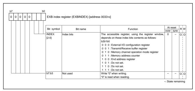
Fig. 111 Structure of EXB index register
