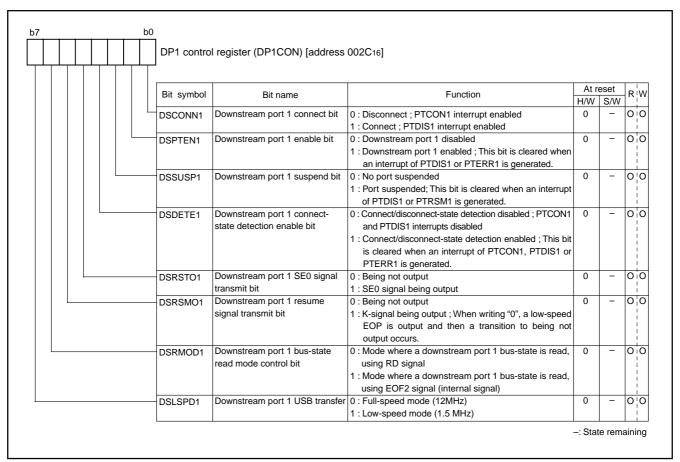
Fig. 97 Structure of DP1 control register
