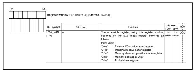
Fig. 112 Structure of Register window 1
