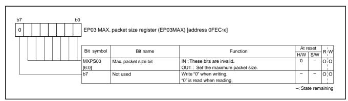
Fig. 72 Structure of EP03 MAX. packet size register
