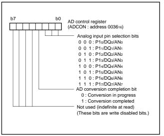
Fig. 132 Structure of AD control register
