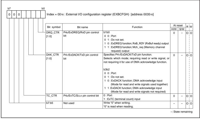
Fig. 115 Index00[high]; Structure of External I/O configuration register
