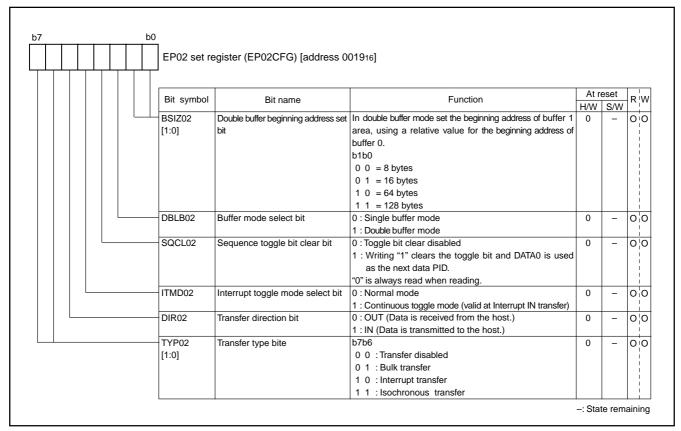
Fig. 56 Structure of EP02 set register
