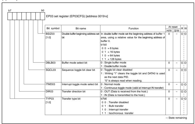
Fig. 65 Structure of EP03 set register
