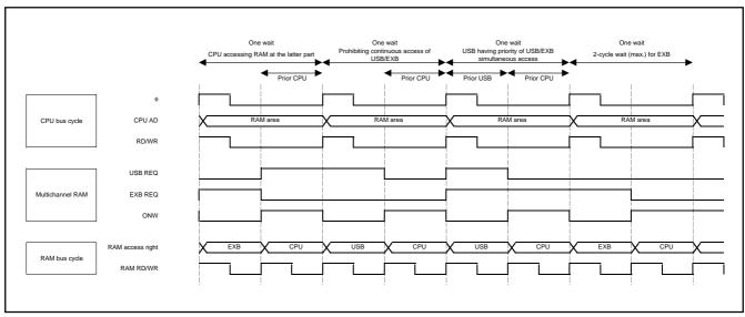
Fig. 130 Multichannel RAM timing diagram (one wait)
