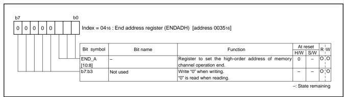
Fig. 121 Index04[high]; Structure of End address register
