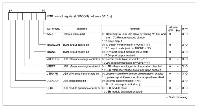
Fig. 31 Structure of USB control register
