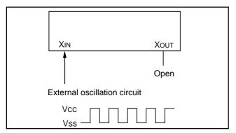
Fig. 142 External clock input circuit
