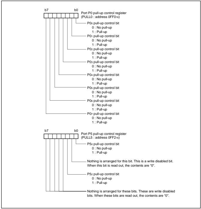
Fig. 12 Structure of port I/O-related registers
