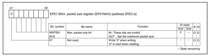
Fig. 54 Structure of EP01 MAX. packet size register
