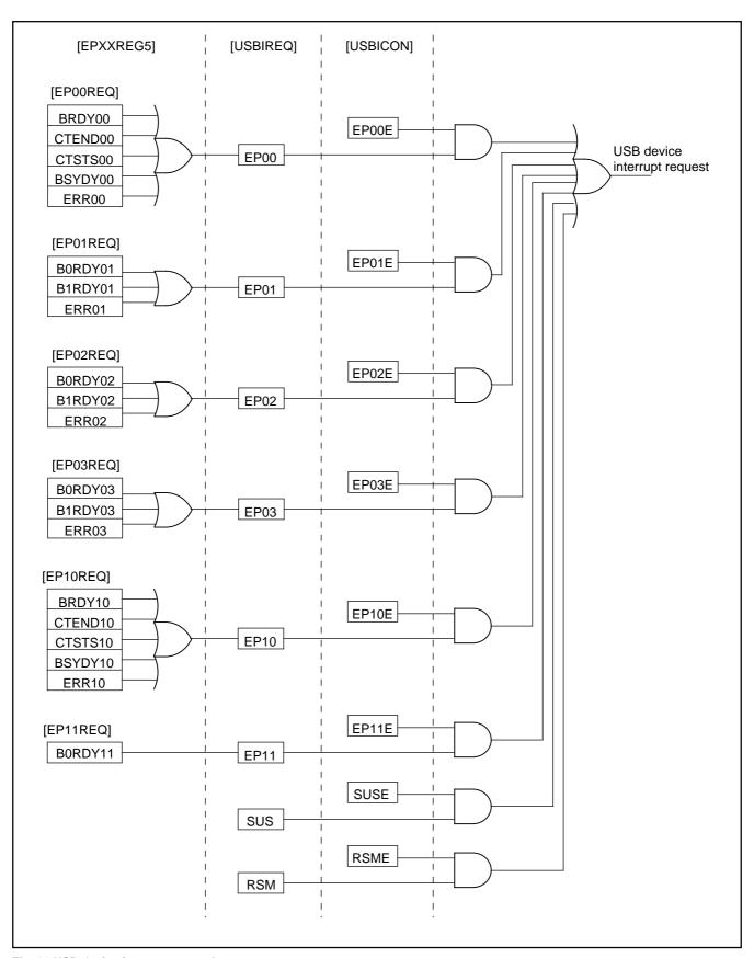
Fig. 29 USB device interrupt control
