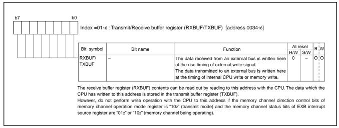
Fig. 116 Index01[low]; Structure of Transmit/Receive buffer register
