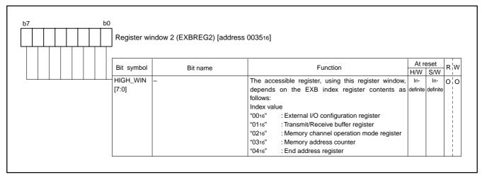
Fig. 113 Structure of Register window 2
