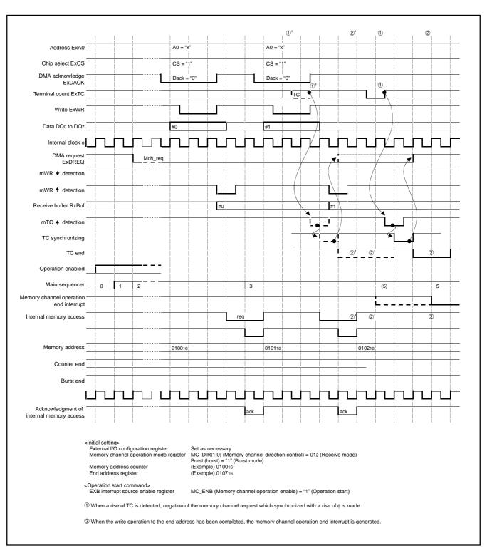
Fig. 126 Memory channel receiving operation (3)
