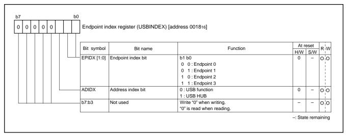
Fig. 39 Structure of Endpoint index register
