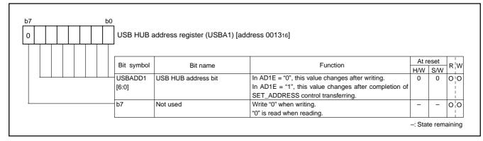
Fig. 34 Structure of USB HUB address register
