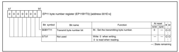
Fig. 85 Structure of EP11 byte number register
