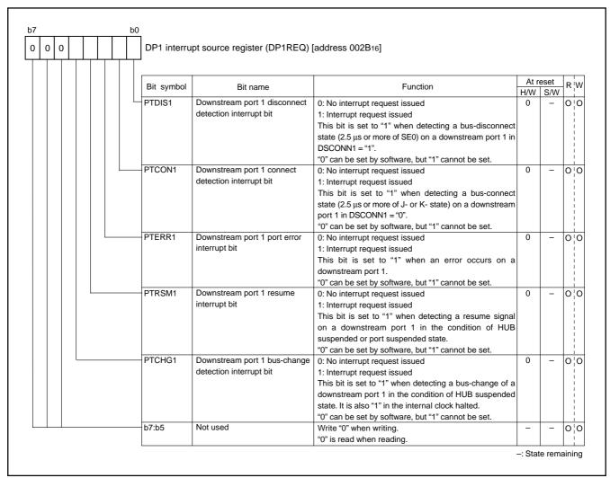
Fig. 96 Structure of DP1 interrupt source register
