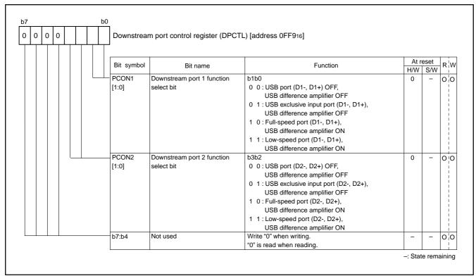
Fig. 102 Structure of Downstream port control register
