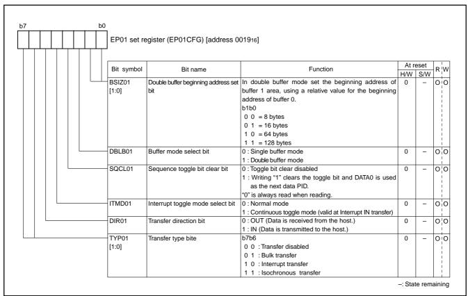
Fig. 47 Structure of EP01 set register
