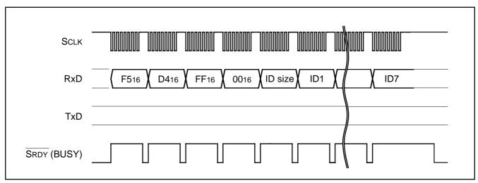
Fig. 163 Timing for ID check
