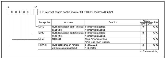
Fig. 93 Structure of HUB interrupt source enable register
