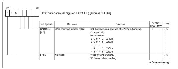
Fig. 73 Structure of EP03 buffer area set register
