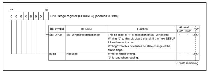
Fig. 40 Structure of EP00 stage register
