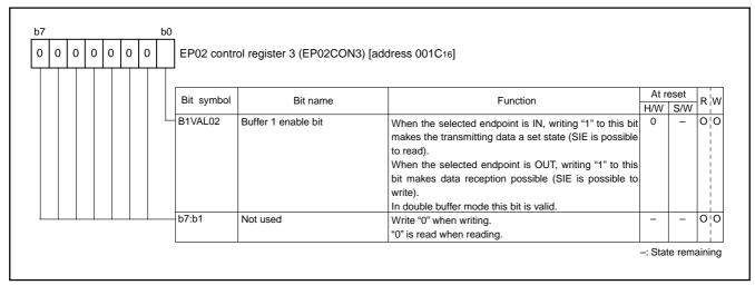
Fig. 59 Structure of EP02 control register 3
