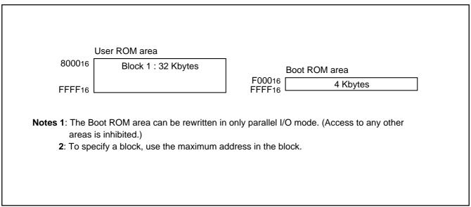
Fig. 146 Block diagram of built-in flash memory
