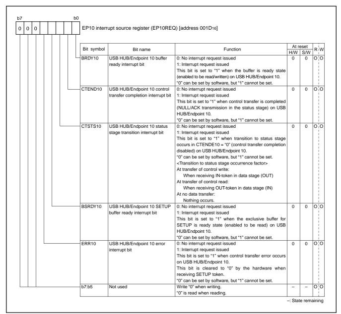
Fig. 78 Structure of EP10 interrupt source register
