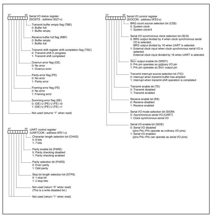
Fig. 22 Structure of serial I/O control registers
