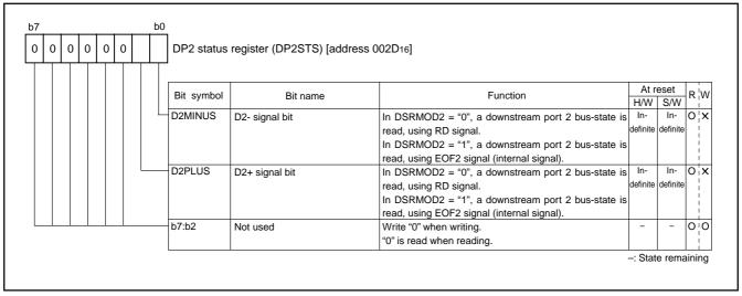
Fig. 101 Structure of DP2 status register
