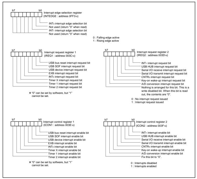
Fig. 14 Structure of interrupt-related registers
