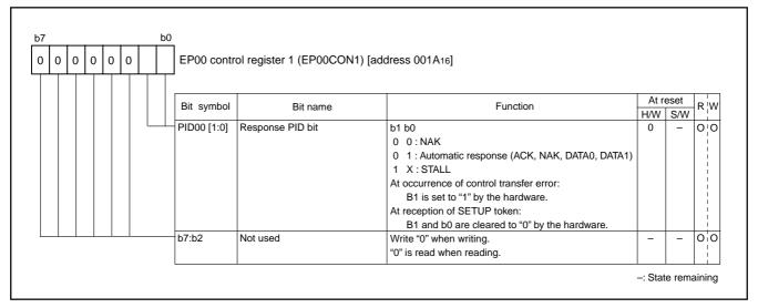
Fig. 41 Structure of EP00 control register 1
