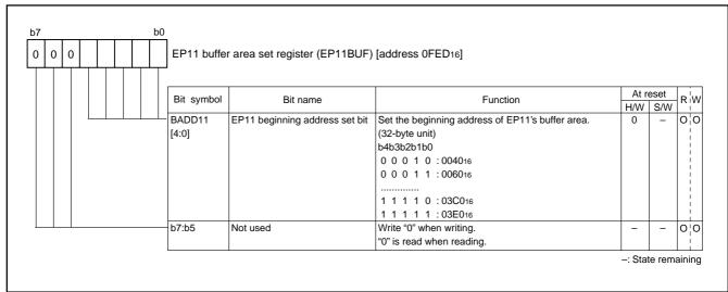
Fig. 86 Structure of EP11 buffer area set register
