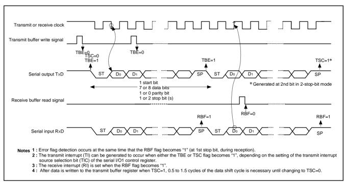
Fig. 21 Operation of UART serial I/O function
