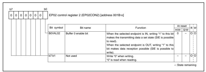
Fig. 58 Structure of EP02 control register 2
