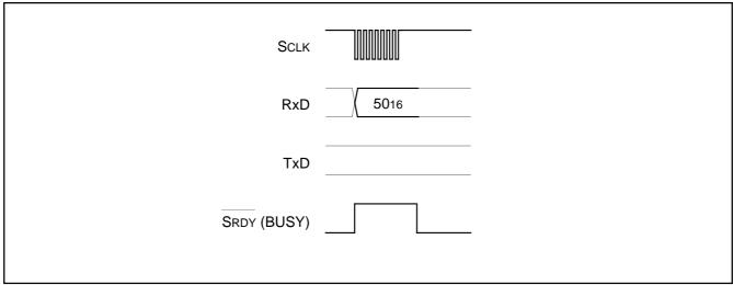
Fig. 157 Timing for clear status register
