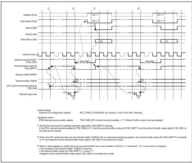
Fig. 123 CPU channel tranmitting operation
