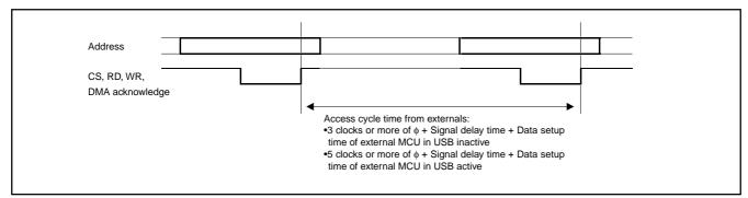
Fig. 104 Data transfer timing of memory channel
