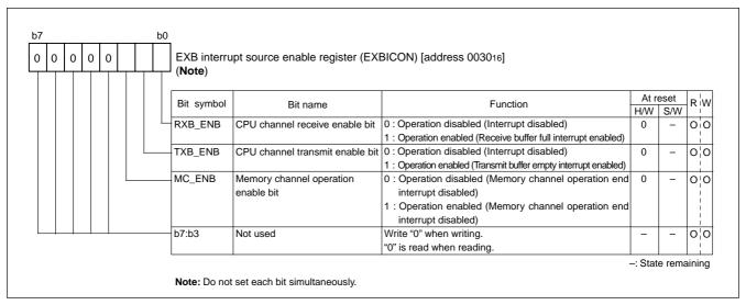
Fig. 109 Structure of EXB interrupt source enable register
