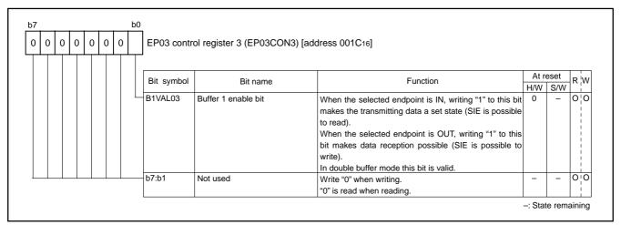
Fig. 68 Structure of EP03 control register 3
