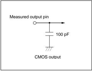
Fig. 168 Output switching characteristics measurement circuit
