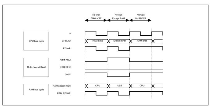
Fig. 129 Multichannel RAM timing diagram (no wait)
