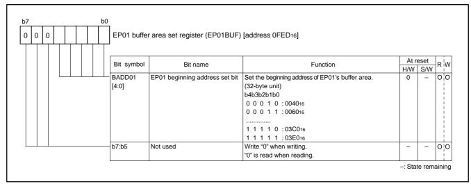
Fig. 55 Structure of EP01 buffer area set register
