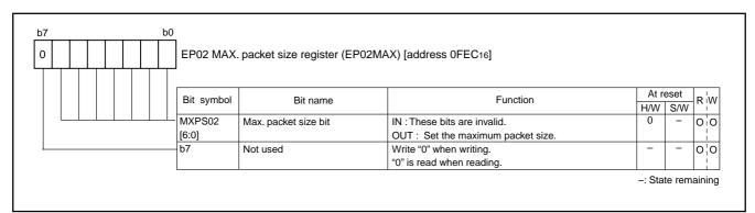
Fig. 63 Structure of EP02 MAX. packet size register
