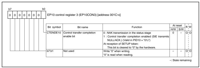
Fig. 77 Structure of EP10 control register 3
