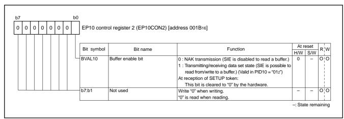
Fig. 76 Structure of EP10 control register 2
