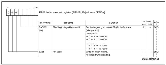
Fig. 64 Structure of EP02 buffer area set register
