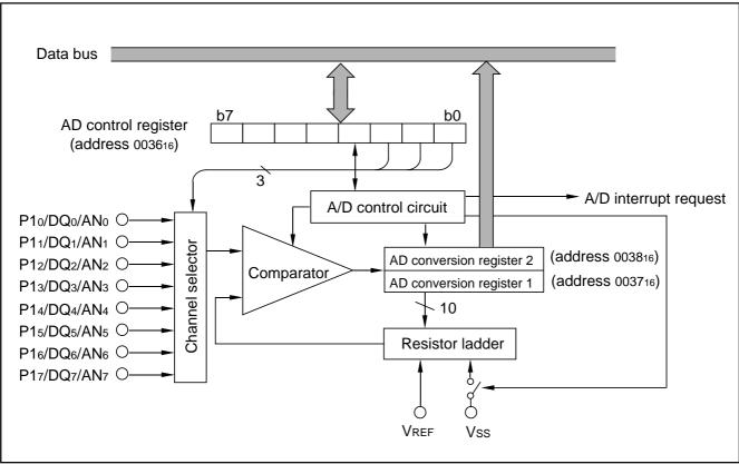
Fig. 134 A/D converter block diagram
