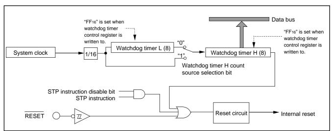
Fig. 135 Block diagram of Watchdog timer
