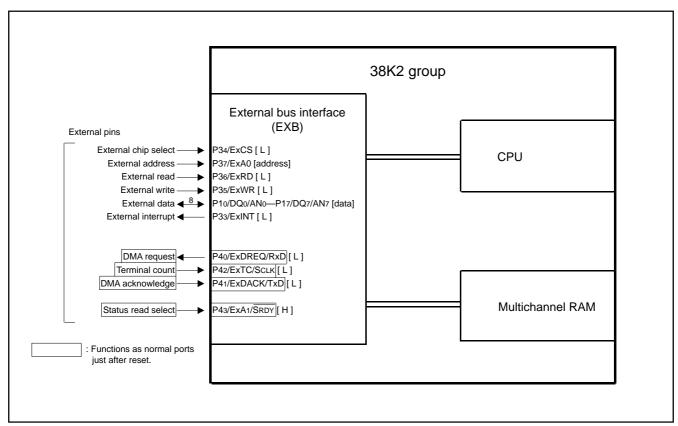
Fig. 105 External bus interface (EXB) pin assignment
