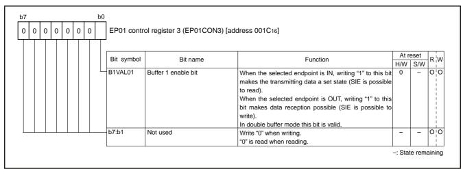
Fig.50 Structure of EP01 control register 3
