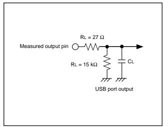
Fig. 169 USB output switching characteristics measurement circuit (1) for D0-, D1+/D2+ (low-speed), D1-/D2- (full-speed)
