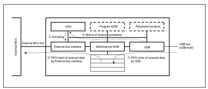
Fig. 131 Multichannel RAM operation example
