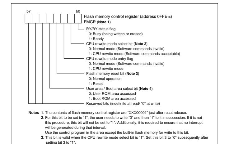
Fig. 147 Structure of flash memory control register
