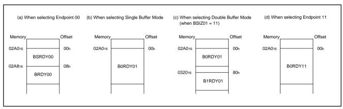
Fig. 28 Examples of interrupt source dependant buffer area offset address
