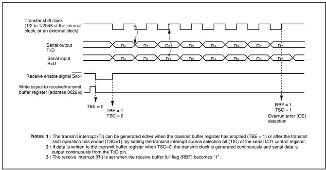
Fig. 19 Operation of clock synchronous serial I/O function
