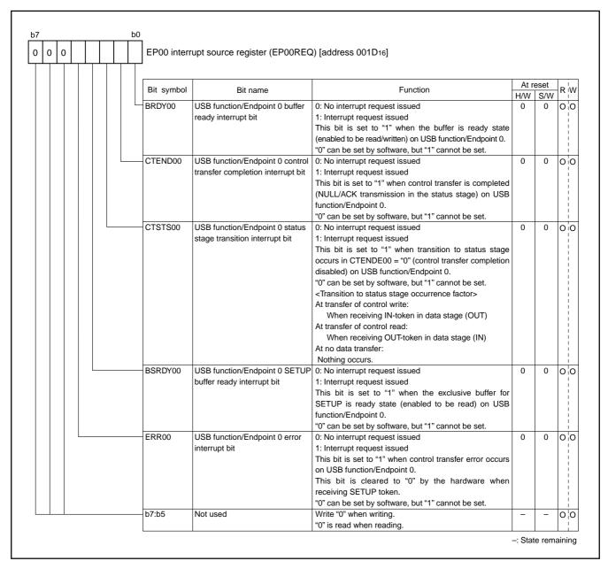
Fig. 44 Structure of EP00 interrupt source register
