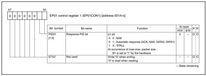
Fig. 48 Structure of EP01 control register 1
