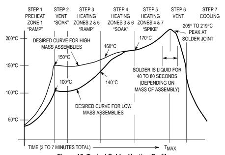
Figure 18. Typical Solder Heating Profile
