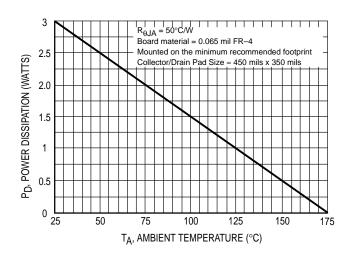
Figure 15. D<sup>2</sup>PAK Power Derating Curve
