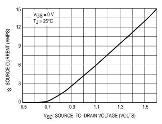
Figure 10. Diode Forward Voltage versus Current
