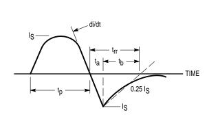
Figure 14. Diode Reverse Recovery Waveform
