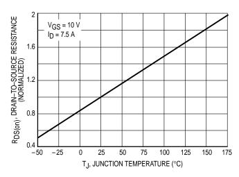
Figure 5. On–Resistance Variation with Temperature
