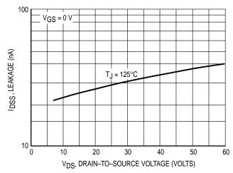
Figure 6. Drain-To-Source Leakage Current versus Voltage
