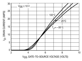
Figure 2. Transfer Characteristics
