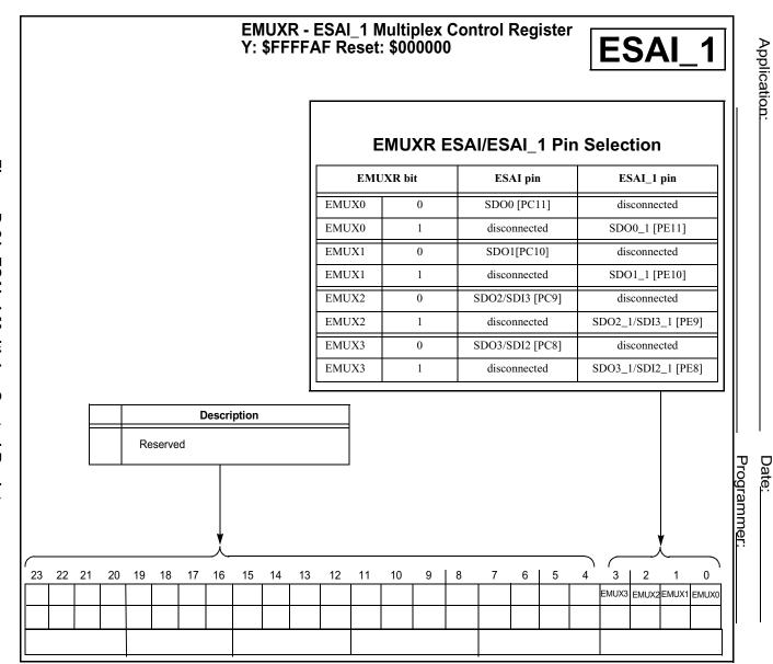
Figure D-21 ESAI\_1 Multiplex Control Register
