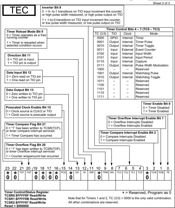
Figure D-31 Timer Control/Status Register
