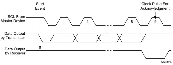
Figure 7-9 Acknowledgment on the I<sup>2</sup>C Bus
