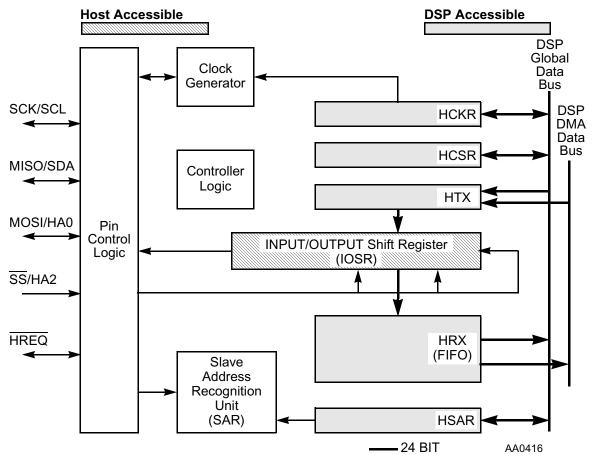
Figure 7-1 Serial Host Interface Block Diagram
