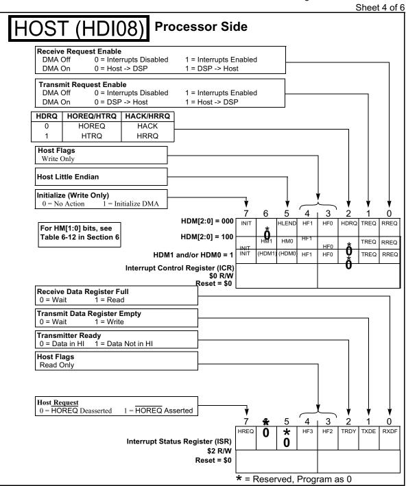
Figure D-9 Host Interrupt Control and Interrupt Status
