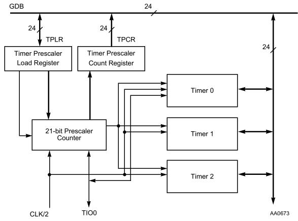
Figure 11-1 Timer/Event Counter Block Diagram
