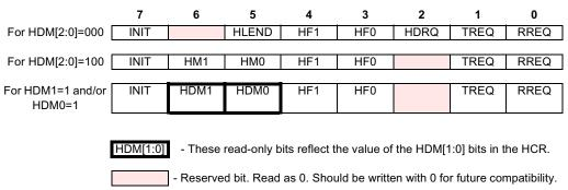
Figure 6-12 Interface Control Register (ICR)
