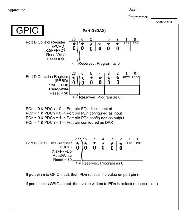
Figure D-35 GPIO Port D
