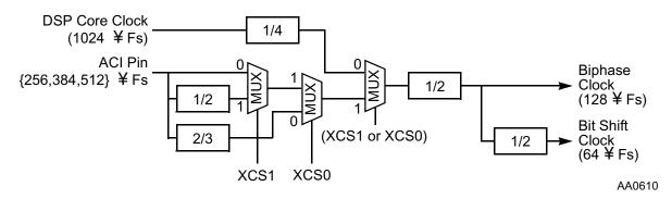
Figure 10-5 Clock Multiplexer Diagram
