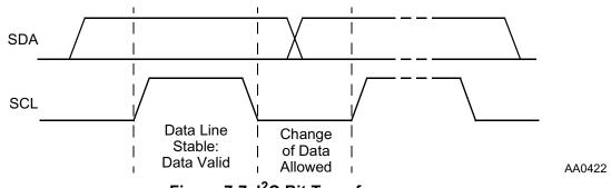
Figure 7-7 I<sup>2</sup>C Bit Transfer
