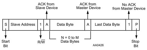
Figure 7-11 I<sup>2</sup>C Bus Protocol For Host Read Cycle
