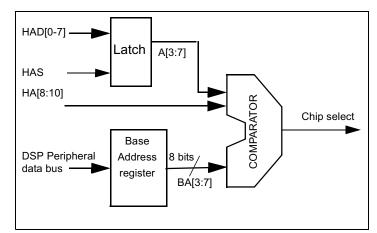
Figure 6-5 Self Chip Select logic
