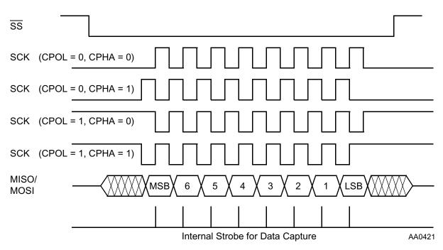
Figure 7-6 SPI Data-To-Clock Timing Diagram
