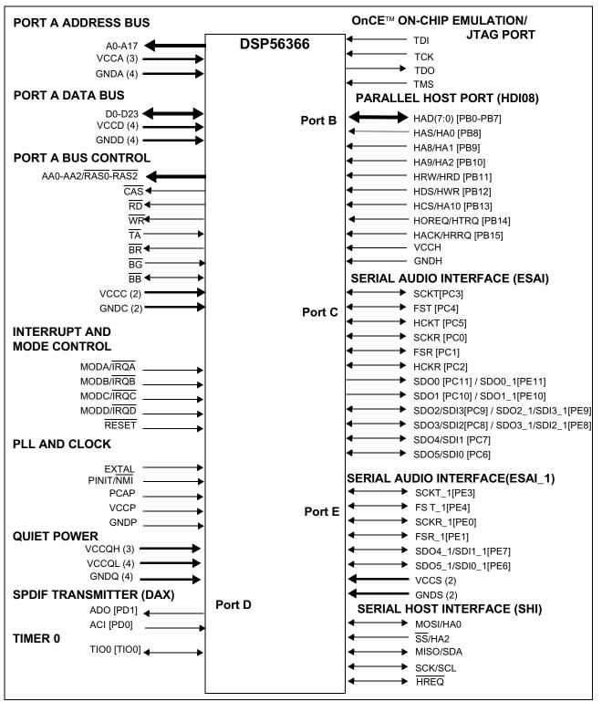
Figure 2-1 Signals Identified by Functional Group
