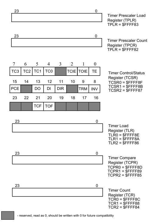
Figure 11-3 Timer Module Programmer's Model
