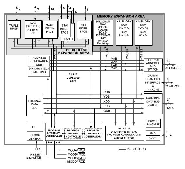
Figure 1-1 DSP56366 Block Diagram
