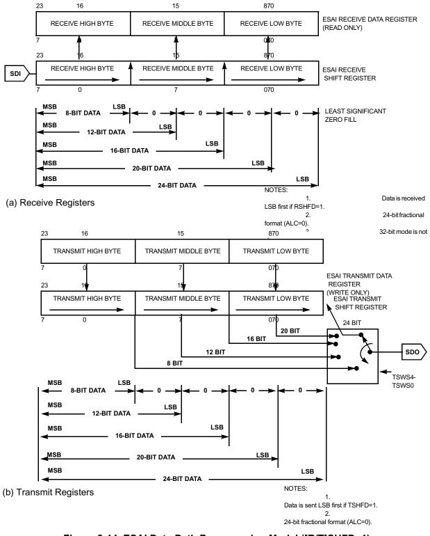
Figure 8-14 ESAI Data Path Programming Model ([R/T]SHFD=1)
