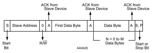
Figure 7-10 I<sup>2</sup>C Bus Protocol For Host Write Cycle
