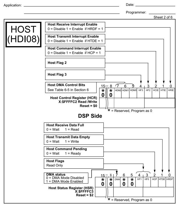
Figure D-7 Host Control and Status Registers
