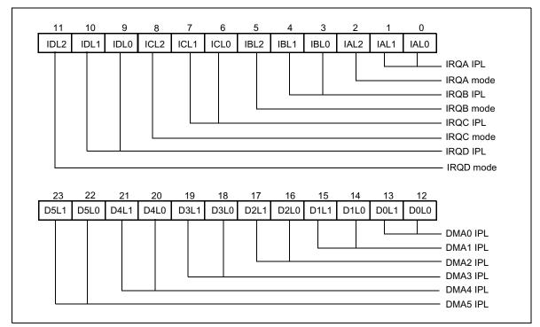
Figure 4-2 Interrupt Priority Register C
