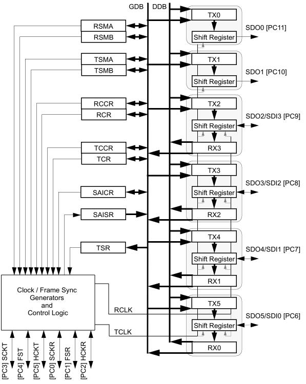
Figure 8-1 ESAI Block Diagram
