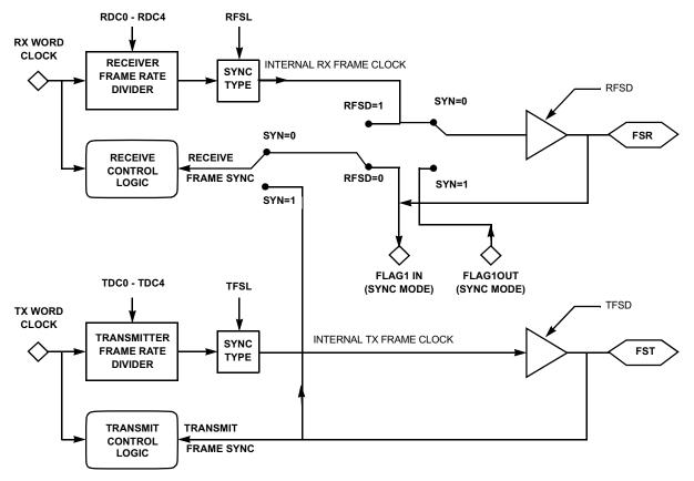
Figure 8-4 ESAI Frame Sync Generator Functional Block Diagram
