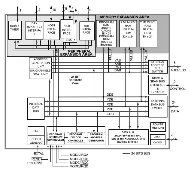
Figure 1-1 DSP56366 Block Diagram
