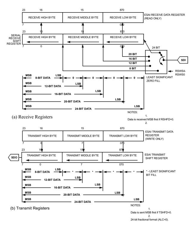
Figure 8-13 ESAI Data Path Programming Model ([R/T]SHFD=0)
