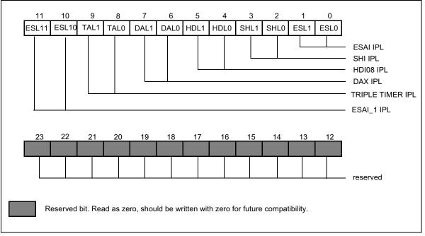
Figure 4-1 Interrupt Priority Register P
