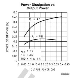
**Power Dissipation vs Output Power** 0.35 0.3  $= 4 \Omega$ POWER DISSIPATION (W) 0.25 0.2 = 80 0.15 0.1 = 2.6 V $V_{DD}$ 0.05 f = 1 kHzTHD + N  $\leq$  1% 0 0.25 0 0.05 0.1 0.15 0.2 OUTPUT POWER (W)
