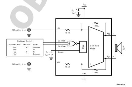
FIGURE 1. Typical Audio Amplifier Application Circuit
