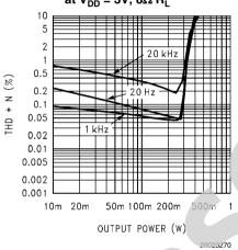
THD+N vs Output Power  $V_{DD} = 3V, \, 4\Omega \; R_L$
