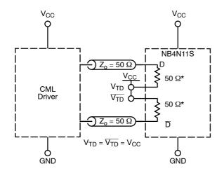
Figure 9. Standard 50  $\Omega$  Load CML Interface
