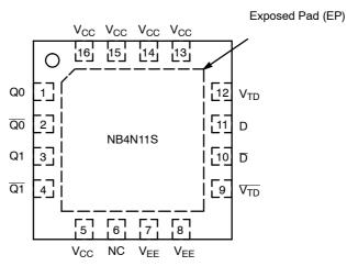
Figure 3. NB4N11S Pinout, 16-pin QFN (Top View)
