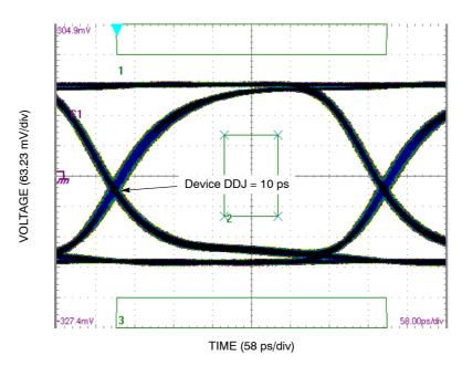
Figure 5. Typical Output Waveform at 2.488 Gb/s with PRBS  $2^{23-1}$  and OC48 mask (V<sub>INPP</sub> = 100 mV; Input Signal DDJ = 14 ps)
