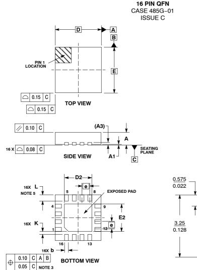
NOTES: 1. DIMENSIONING AND TOLERANCING PER ASME Y14 5M 1994
