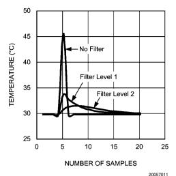
FIGURE 7. Impulse Response of the Digital Filter
