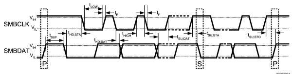
**SMBus Timing Diagram for SMBCLK and SMBDAT Signals**
