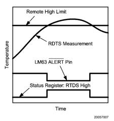
FIGURE 3. ALERT Output as Temperature Comparator Response Diagram
