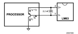
FIGURE 10. Processor Connection to LM63
