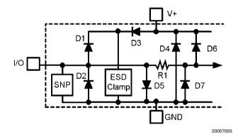
**FIGURE 1. ESD Protection Input Structure**
