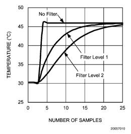
FIGURE 6. Step Response of the Digital Filter
