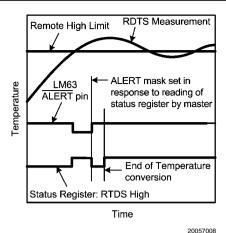
FIGURE 4. ALERT Output as an Interrupt Temperature
