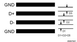
FIGURE 12. Ideal Diode Trace Layout
