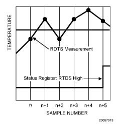
FIGURE 9. Fault Queue Temperature Response Diagram
