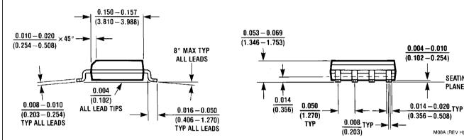
8-Lead (0.154-Inch Wide) Molded Narrow Small-Outline Package (SOIC) JEDEC Registration Number MS-012 Order Number LM63CIM **NS Package Number M008A**
