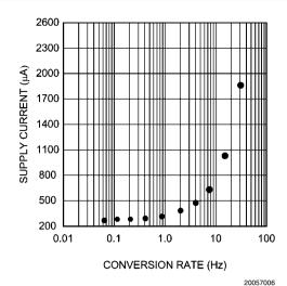
FIGURE 2. Supply Current vs Conversion Rate
