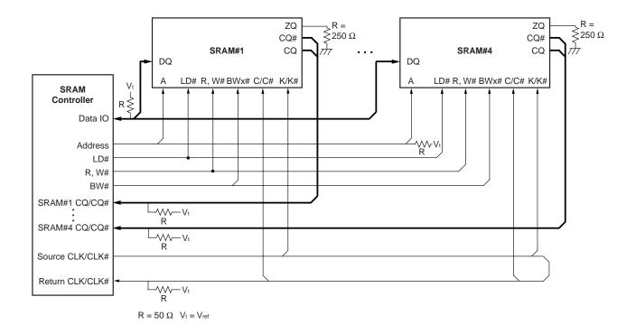
**Remark** AC Characteristics are defined at the condition of SRAM outputs, CQ, CQ# and DQ with termination.
