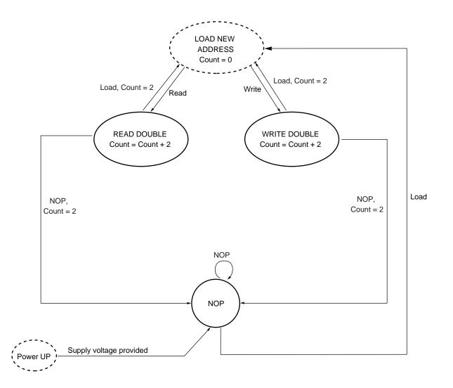
**Remarks 1.** A0 is internally advanced in accordance with the burst order table. Bus cycle is terminated after burst count = 2.
