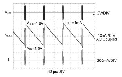
Figure 14. Typical ECO Operation
