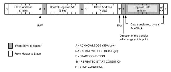
Figure 19. Register Read Format
