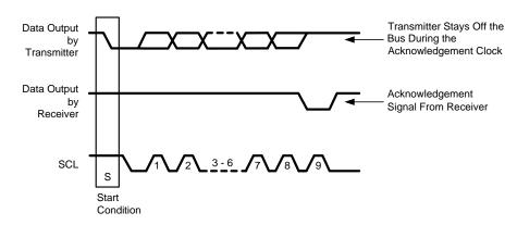
Figure 17. Bus Acknowledge Cycle
