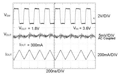
Figure 13. Typical PWM Operation
