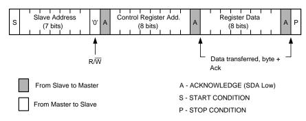
Figure 18. Register Write Format
