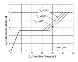
Figure 6. Gate Charge Characteristics
