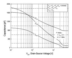
Figure 5. Capacitance Characteristics
