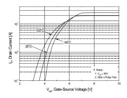
Figure 2. Transfer Characteristics
