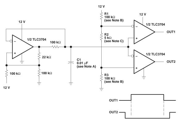
NOTES: A. Adjust C1 for a change in oscillator frequency where:  $1/f = 1.85(100 \; k\Omega)C1$
