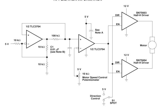
NOTES: A. The recommended minimum capacitance is 10  $\mu\text{F}$  to eliminate common ground switching noise.
