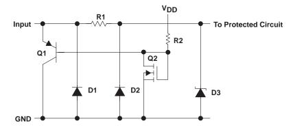
Figure 1. LinCMOS ESD-Protection Schematic
