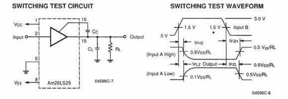
Figure 2. Three-State Delays
