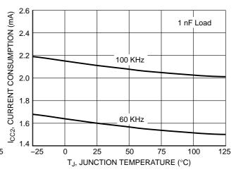
Figure 5. IC Current Consumption, I<sub>CC1</sub> vs. Junction Temperature
