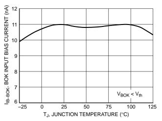
Figure 24. BOK Input Bias Current vs. Junction Temperature
