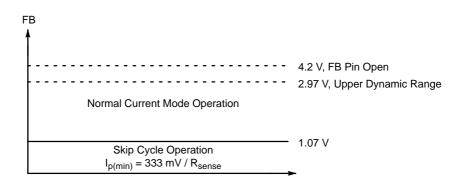
Figure 29. Feedback Pin Voltage and Modes of Operation
