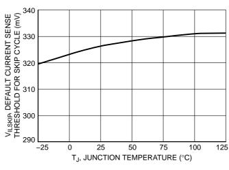
Figure 15. Default Current Setpoint for Skip Cycle vs. Junction Temperature
