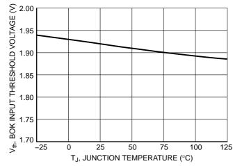
Figure 23. BOK Threshold Voltage vs. Junction Temperature
