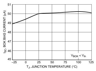
Figure 25. BOK Source Bias Current vs. Junction Temperature
