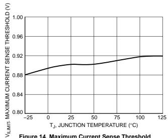
Figure 14. Maximum Current Sense Threshold vs. Junction Temperature
