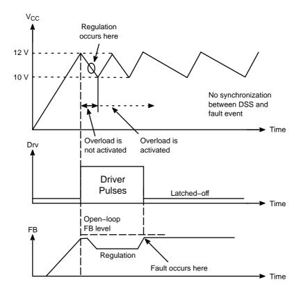
Figure 34. Fault Protection Timing Diagram
