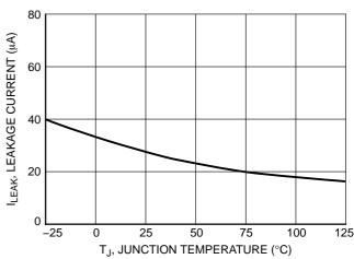
Figure 10. Leakage Current vs. Junction Temperature
