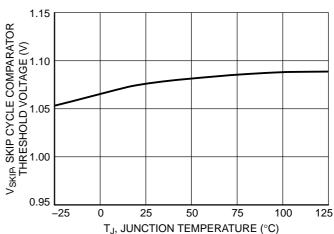
Figure 26. Skip Mode Threshold Voltage vs. Junction Temperature
