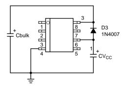
Figure 37. or a diode forces V<sub>CC</sub> to reach UVLOlow sooner
