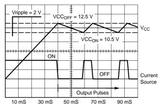
Figure 27. The Charge/Discharge Cycle Over a 10  $\mu$ F V<sub>CC</sub> Capacitor
