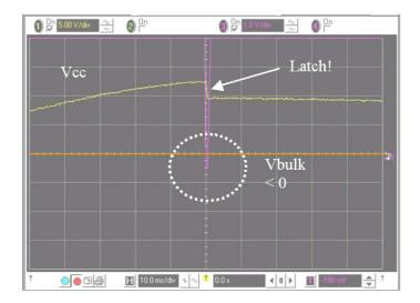
Figure 35. A negative spike takes place on the Bulk capacitor at the switch-off sequence
