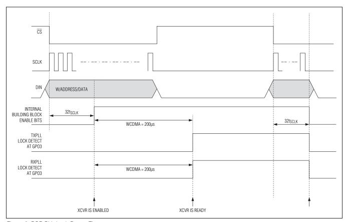
Figure 3. POR PLL Lock-Detect Time
