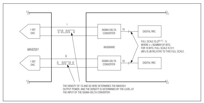
Figure 2. Baseband Input Example
