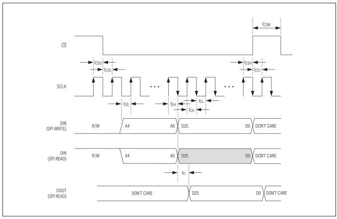
Figure 4. SPI Timing
