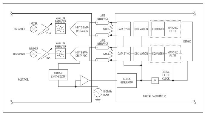
Figure 1. Digital Baseband Receiver Interface
