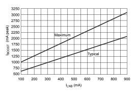
Figure 4. Boost inductor peak current versus  $I_{LNB}$
