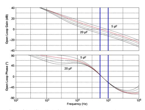
Figure 7. Gain and Phase Margin of the boost loop at various capacitance values
