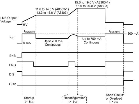
Figure 1. Startup, Reconfiguration, and Short Circuit operation using R  $_{\text{SET}}$  = 37.4 k $\Omega,$  and a capacitive load
