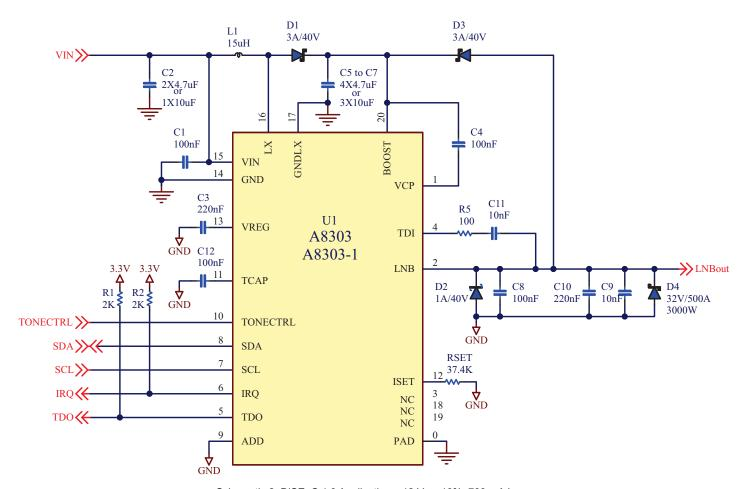
Schematic 2. DiSEqC 1.0 Applications, 12 V<sub>IN</sub> ±10%, 700 mA I<sub>OUT</sub>, surge of ±1000 V, 2  $\Omega$ , 1.2/50  $\mu s$  – 8/20  $\mu s$  combination wave
