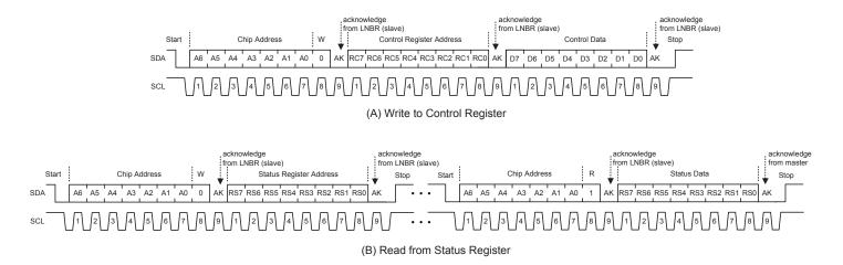
Figure 8. I<sup>2</sup>C™ Interface Read and Write Sequences. (A) for the I<sup>2</sup>C™ Write cycle and (B) for the I<sup>2</sup>C™ Read cycle
