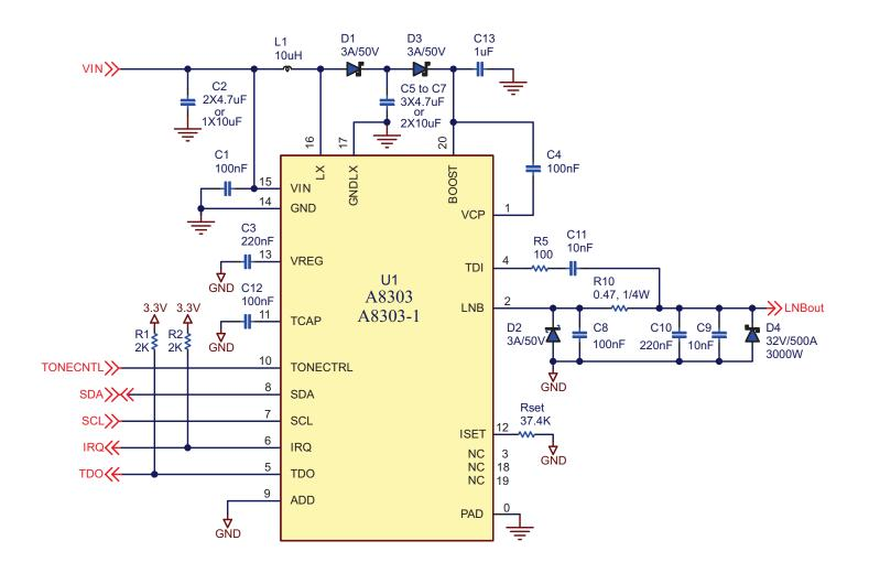
Schematic 4. DiSEqC 1.0 Applications for increased surge requirements  $\pm 1000$  V, 2  $\Omega$ , 1.2/50  $\mu$ s – 8/20  $\mu$ s combination wave, and "stress to TVS failure" (or  $\pm 4000$  V) test
