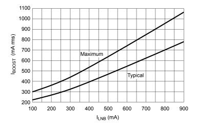
Figure 5. Boost capacitor rms current versus I<sub>LNB</sub>
