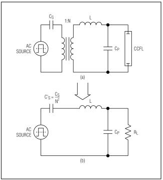
Figure 5. Equivalent Resonant Tank Circuit
