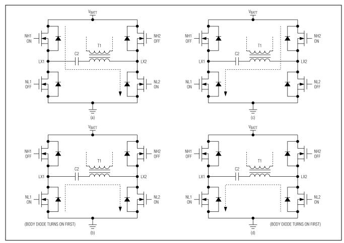
Figure 4. Resonant Operation
