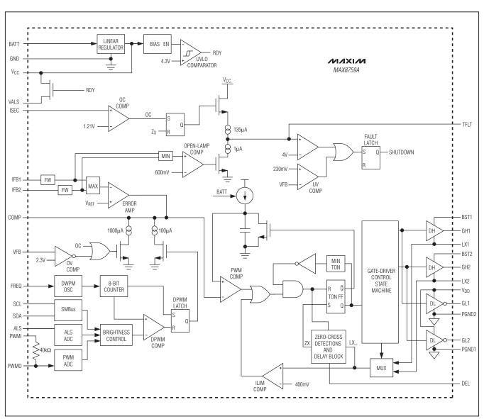
Figure 2. MAX8759A Functional Diagram
