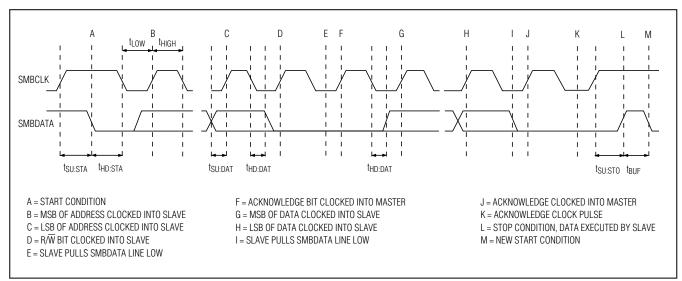
Figure 9. SMBus Write Timing
