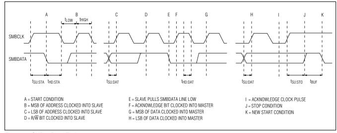
Figure 10. SMBus Read Timing
