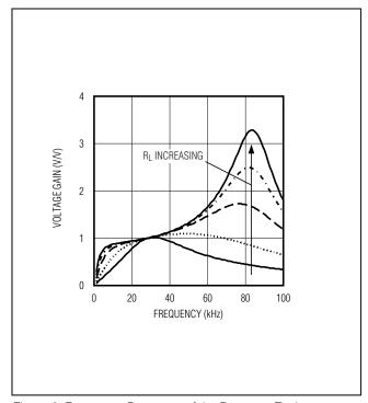
Figure 6. Frequency Response of the Resonant Tank
