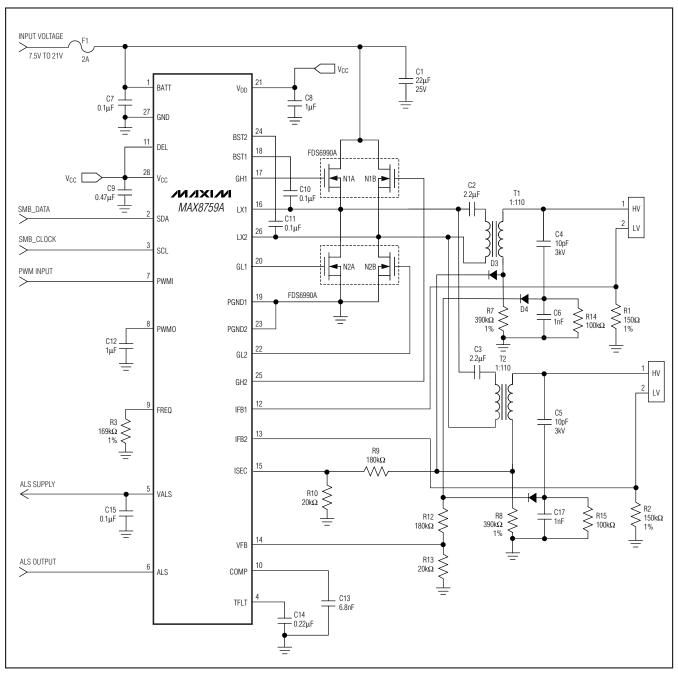
Figure 11. Typical MAX8759A Dual-Lamp Operating Circuit
