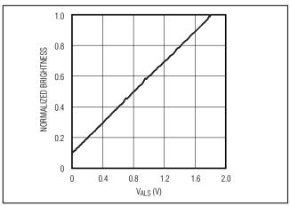
Figure 7. Normalized Brightness vs. ALS Voltage
