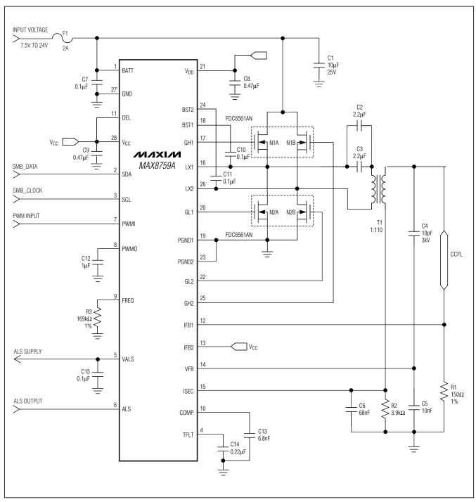
Figure 1. Typical MAX8759A Single-Lamp Operating Circuit
