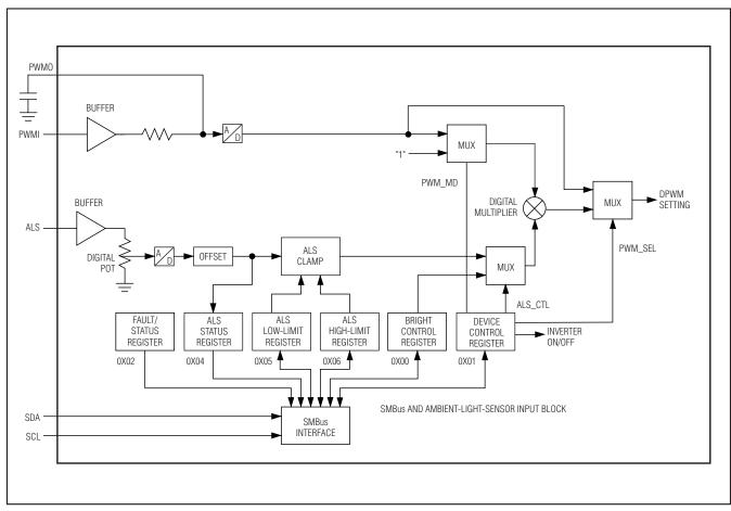
Figure 3. MAX8759A SMBus and Ambient-Light-Sensor Input Block
