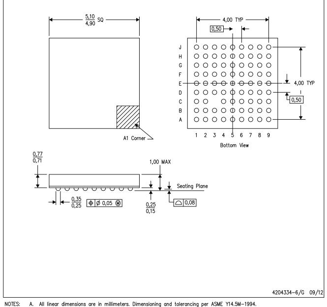
A. All linear almensions are in millimeters. Dimensioning and toil
