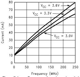
Figure 7. I<sub>CC</sub> vs Frequency, four channels switching
