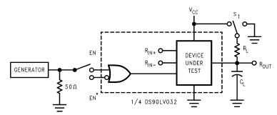
$\rm C_L$  includes load and test jig capacitance.
