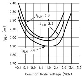
Figure 11. Variation in Low to High Propagation Delay versus V<sub>CM</sub>
