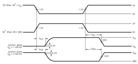
Figure 6. Receiver TRI-STATE Delay Waveforms
