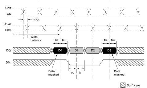
Figure 2-7. Basic WRITE Burst / DM Timing
