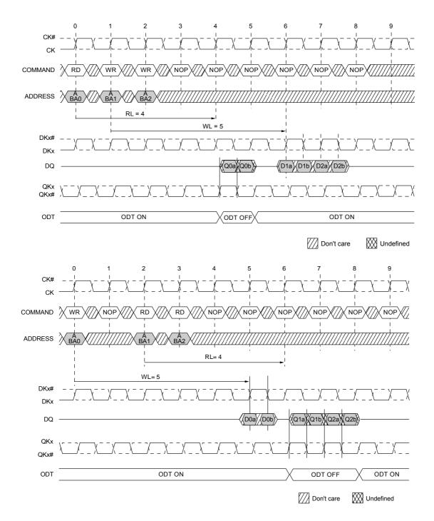
Figure 2-24. READ followed by WRITE with ODT: BL=2, Configuration 1
