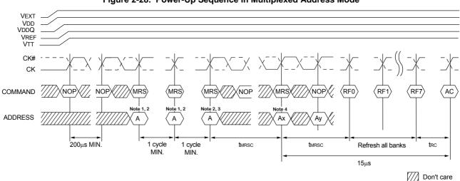
Figure 2-28. Power-Up Sequence in Multiplexed Address Mode
