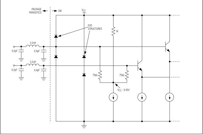
Figure 3. MAX3752 Input Structure
