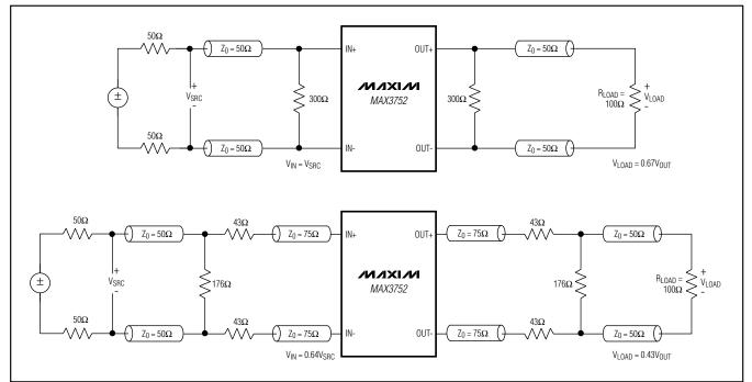
Figure 5. Interfaces to 50 $\Omega$  Systems
