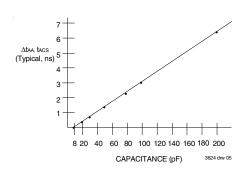
Figure 3. Output Capacitive Derating
