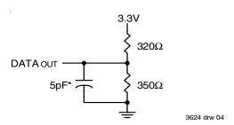
\*Including jig and scope capacitance.
