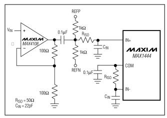
Figure 9. Single-Ended AC-Coupled Input
