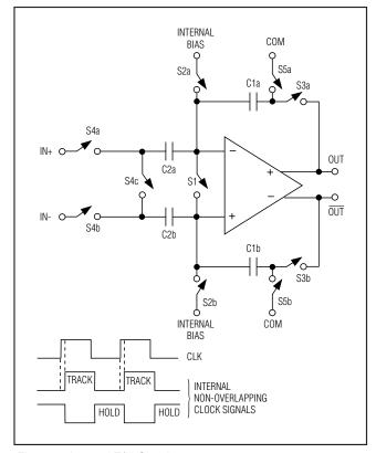
Figure 2. Internal T/H Circuit
