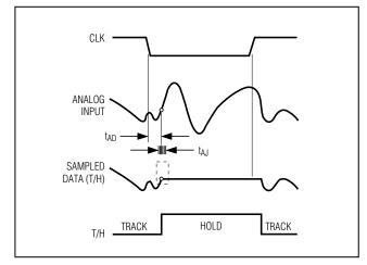
Figure 12. T/H Aperture Timing
