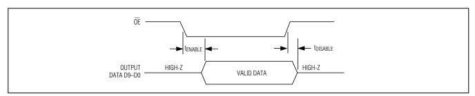
Figure 5. Output Enable Timing
