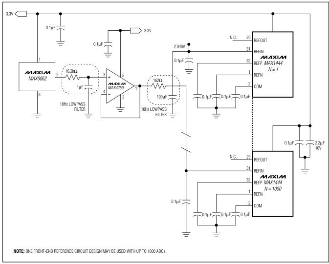
Figure 10. Buffered External Reference Drives Up to 1000 ADCs
