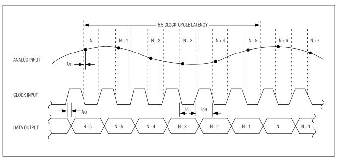
Figure 6. System and Output Timing Diagram
