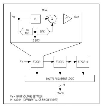
Figure 1. Pipelined Architecture—Stage Blocks
