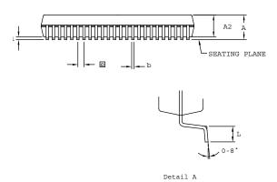
Figure 63. 48-Pin SSOP Package Design
