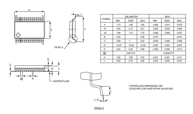
Figure 62. 28-Pin SSOP Package Diagram
