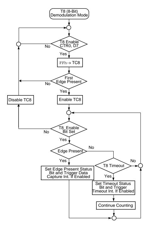
Figure 21. DEMODULATION Mode Flowchart
