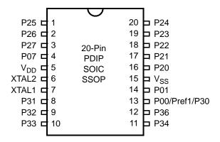
Figure 3. 20-Pin PDIP/SOIC/SSOP Pin Configuration
