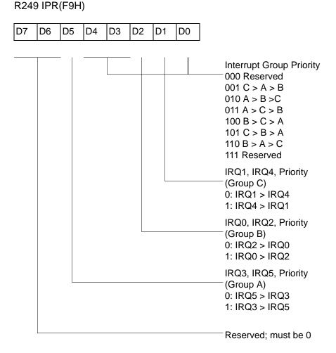
Figure 48.Interrupt Priority Register (F9H: Write Only)
