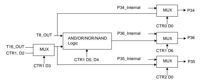
**Figure 26.Output Circuit**
