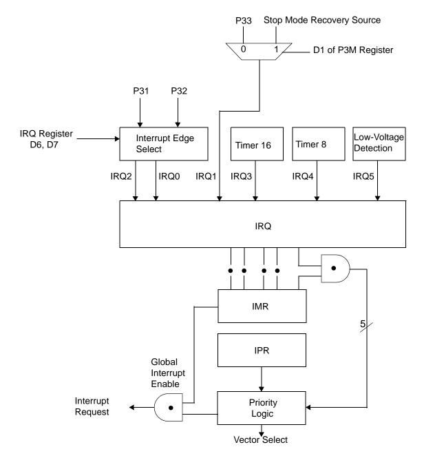
Figure 27. Interrupt Block Diagram
