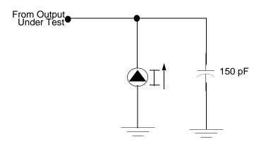
Figure 55.Test Load Diagram
