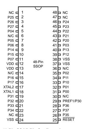
Figure 5. 48-Pin SSOP Pin Configuration
