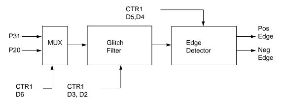
Figure 15.Glitch Filter Circuitry
