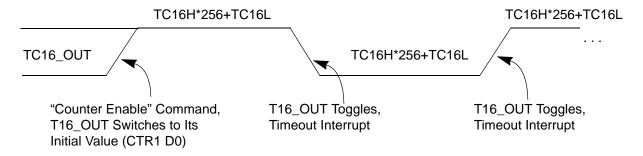
Figure 24.T16\_OUT in Modulo-N Mode
