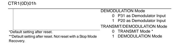
Figure 37.T8 and T16 Common Control Functions ((0D)01H: Read/Write)
