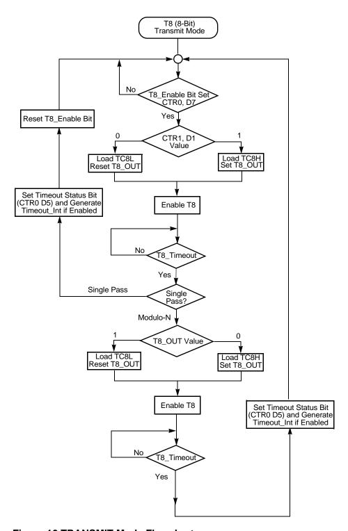
Figure 16.TRANSMIT Mode Flowchart
