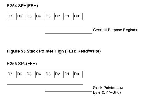
Figure 54.Stack Pointer Low (FFH: Read/Write)
