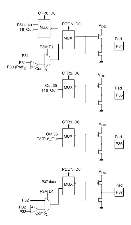
Figure 10. Port 3 Counter/Timer Output Configuration
