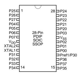
Figure 4. 28-Pin PDIP/SOIC/SSOP Pin Configuration
