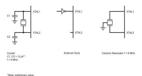
Figure 28.Oscillator Configuration
