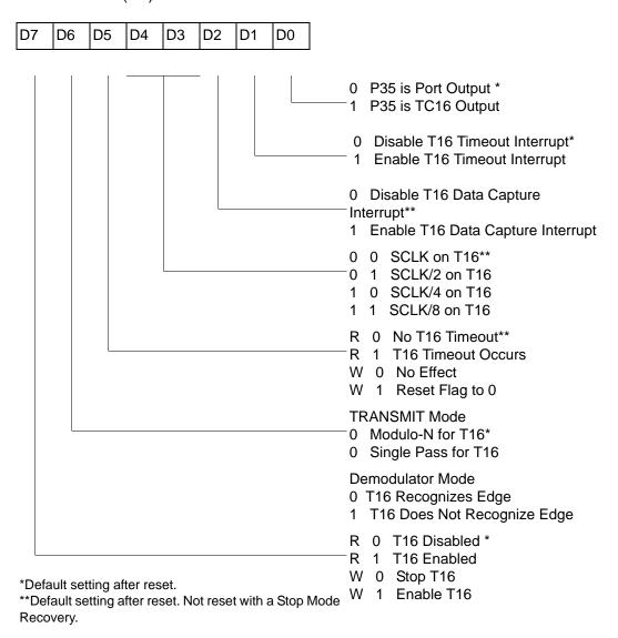
Figure 38. T16 Control Register ((0D) 2H: Read/Write Except Where Noted)
