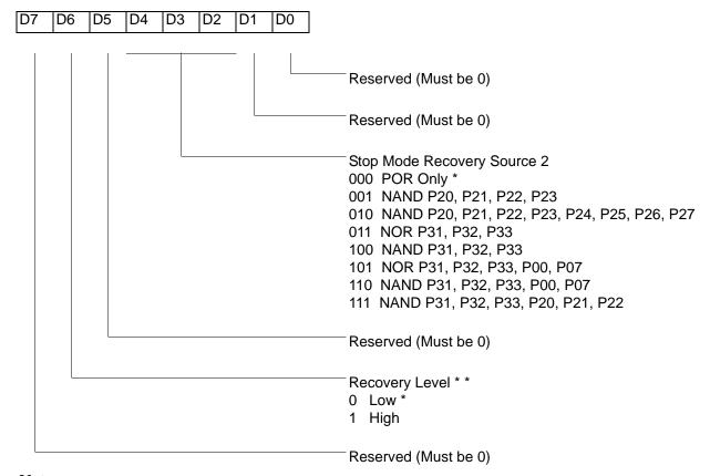
**Note:** If used in conjunction with SMR, either of the two specified events causes a Stop Mode Recovery.
