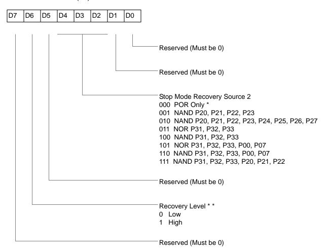
Note: If used in conjunction with SMR, either of the two specified events causes a Stop Mode Recovery.
