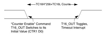
Figure 23.T16 OUT in SINGLE-PASS Mode
