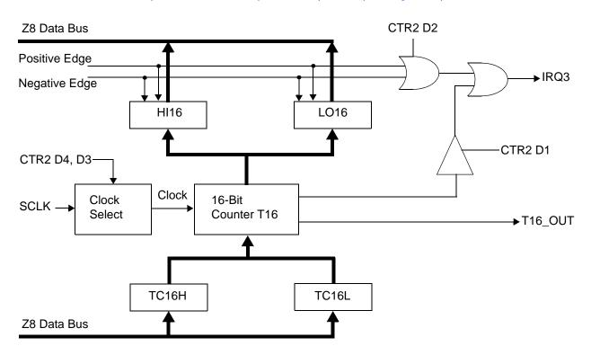
Figure 22.16-Bit Counter/Timer Circuits
