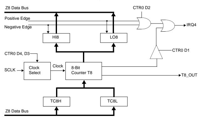
Figure 17.8-Bit Counter/Timer Circuits
