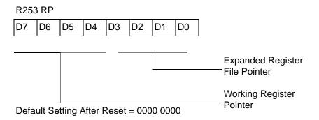
Figure 13. Register Pointer
