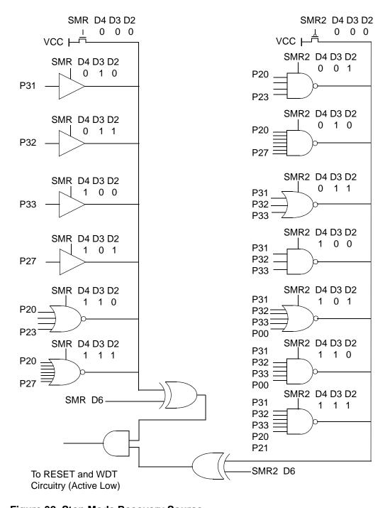
Figure 32. Stop Mode Recovery Source
