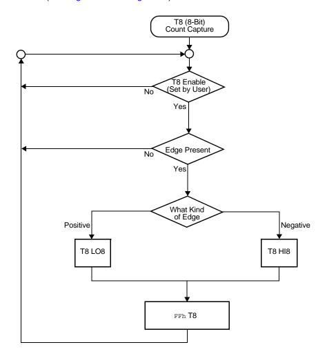
Figure 20.DEMODULATION Mode Count Capture Flowchart
