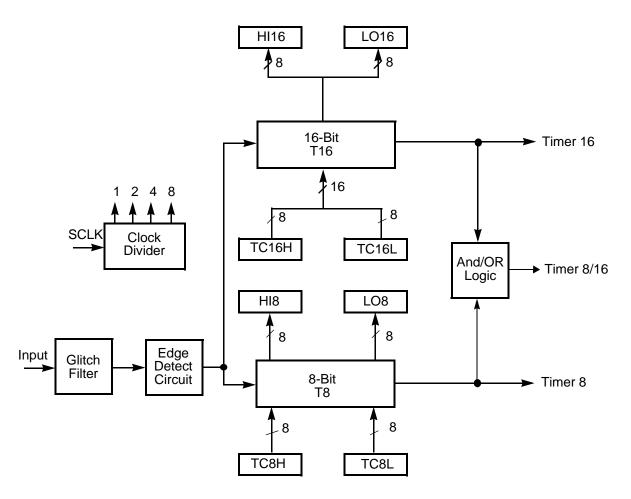
Figure 2. Counter/Timers Diagram
