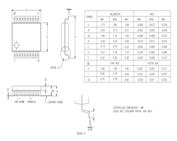
Figure 59. 20-Pin SSOP Package Diagram
