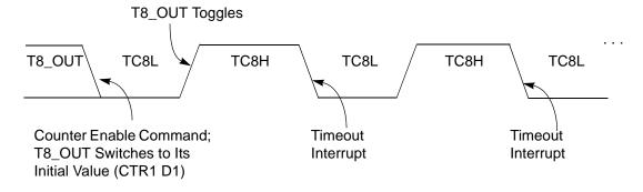
Figure 19. T8\_OUT in MODULO-N Mode
