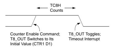
Figure 18. T8\_OUT in SINGLE-PASS Mode
