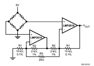
FIGURE 4. Precision Strain Gauge Amplifier
