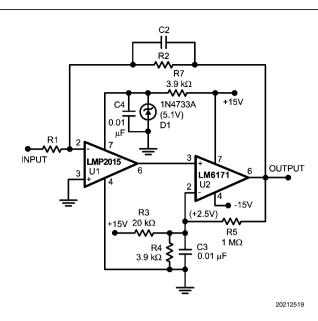
FIGURE 5. Composite Amplifier Configuration
