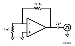
**FIGURE 1. Overload Recovery Test**
