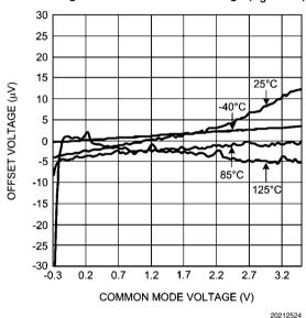
Offset Voltage vs. Common Mode Voltage ( $V_S = +2.7V$ )
