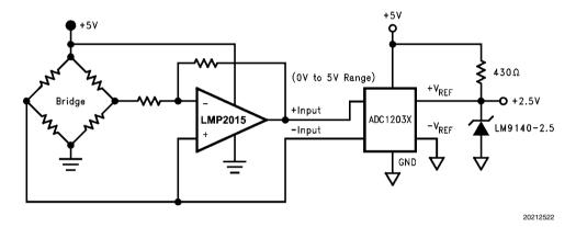
FIGURE 8. DC Coupled ADC Driver
