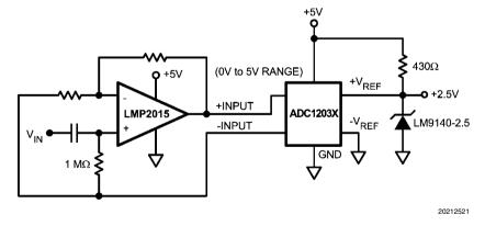
FIGURE 7. AC Coupled ADC Driver
