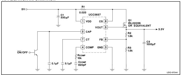
Figure 1. Typical Application 5V to 3.3V, 5A Regulator
