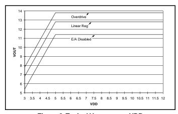
Figure 2. Typical Voutmax vs. VDD
