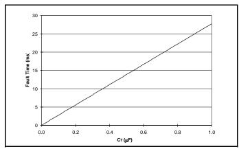
Figure 5. Fault Time vs. Timing Capacitance
