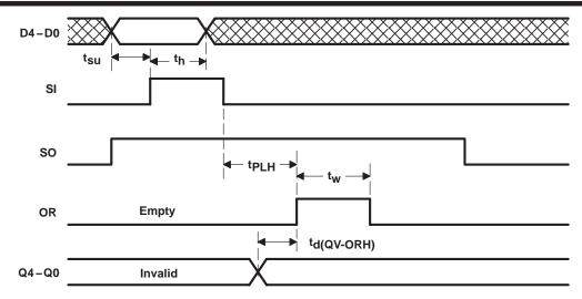
Figure 3. Data Fall-Through Waveforms
