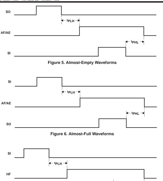
Figure 7. Half-Full Waveforms
