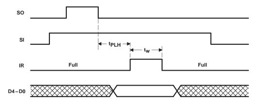
Figure 4. Automatic Data-In Waveforms
