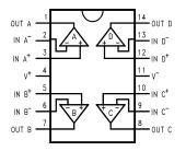
Figure 2. 14-Pin TSSOP See PW Package
