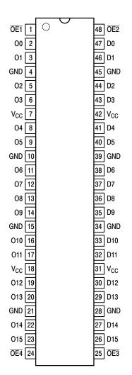
Figure 1. 48-Lead Pinout (Top View)
