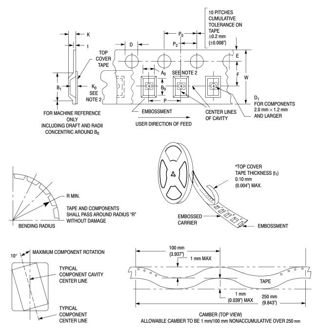
Figure 7. Carrier Tape Specifications
