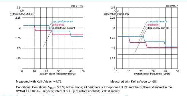
Fig 21. CoreMark score for different power mode settings of the power profiles
