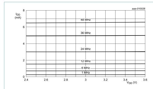
Conditions:  $T_{amb} = 25$  °C; active mode entered executing code while(1)  $\{\}$  from flash; all peripherals disabled in the SYSAHBCLKCTRL register (SYSAHBCLKCTRL = 0x1F), all peripheral clocks disabled; internal pull-up resistors disabled; BOD disabled; low-current mode.
