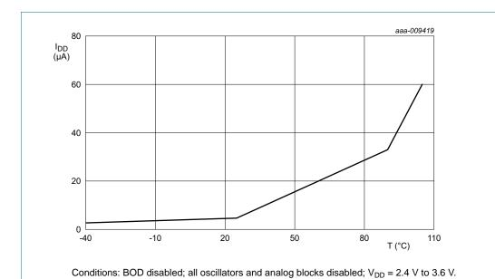
Fig 18. Power-down mode: Typical supply current I<sub>DD</sub> versus temperature for different supply voltages V<sub>DD</sub>
