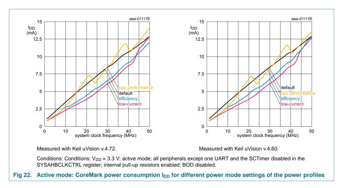
The CoreMark scores serve as a guideline to select the best power mode for a given application. To find the most suitable power mode, run the application in mode and compare power consumption and performance.
