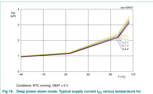
different supply voltages V<sub>DD</sub>
