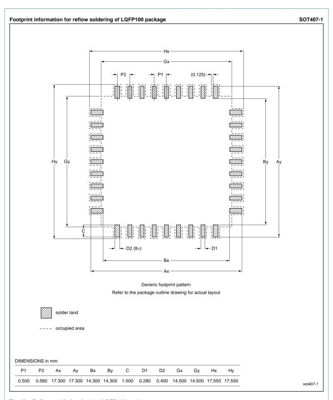
Fig 47. Reflow soldering for the LQFP100 package
