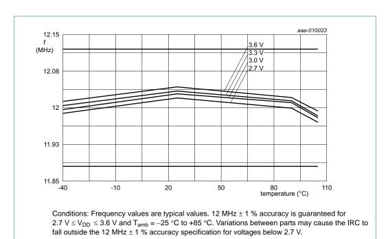
Fig 30. Typical Internal RC oscillator frequency versus temperature
