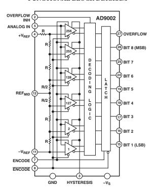
The AD9002 is available in two grades, one with 0.5 LSB linearity and one with 0.75 LSB linearity. Both versions are offered in an industrial grade, -25°C to +85°C, packaged in a 28-lead DIP and a 28-leaded JLCC. The military temperature range devices, -55°C to +125°C, are available in a ceramic DIP package and complies with MIL-STD-883 Class B.
