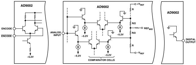
Figure 2. Input/Output Circuits
