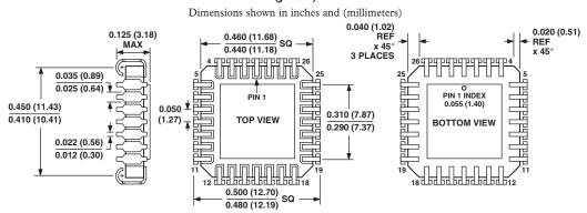
CONTROLLING DIMENSIONS ARE IN INCHES; MILLIMETERS DIMENSIONS (IN PARENTHESES) ARE ROUNDED-OFF INCH EQUIVALENTS FOR REFERENCE ONLY AND ARE NOT APPROPRIATE FOR USE IN DESIGN
