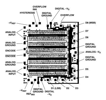
Figure 4. Die Layout and Mechanical Information
