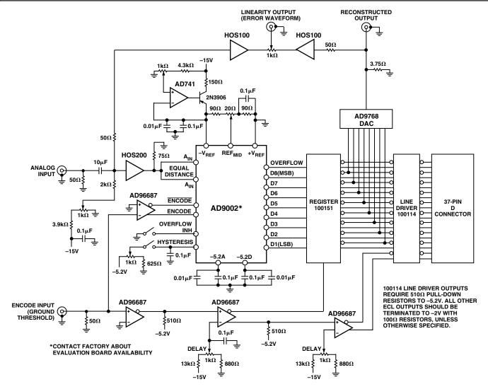
Figure 6. AD9002 Evaluation Circuit
