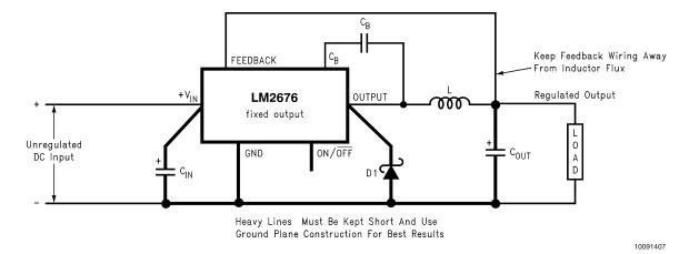
FIGURE 1. Basic circuit for fixed output voltage applications.
