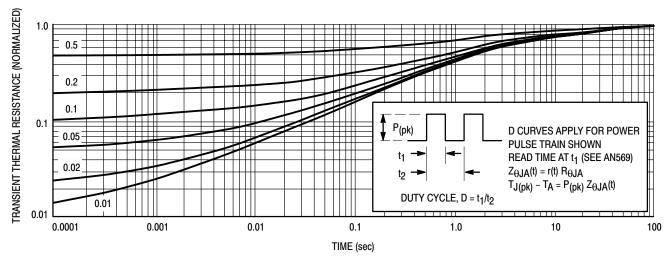
Figure 9. Thermal Response Curve
