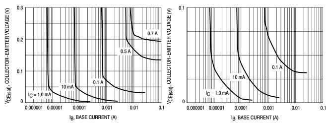
Figure 1. Collector Saturation Region
