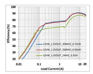
Figure 8. Efficiency vs. Load Current with  $V_{\text{IN}}$ =19 V and  $V_{\text{OUT}}$ =1.2 V
