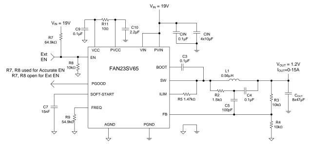
Figure 1. Typical Application with  $V_{IN} = 19 \text{ V}$
