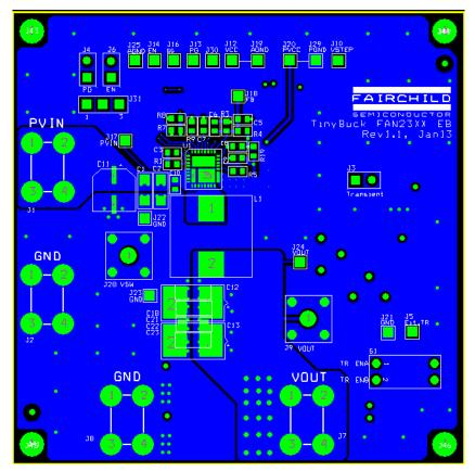
Figure 28. Evaluation Board Top Layer Copper
