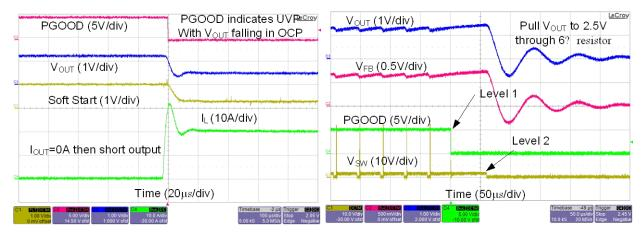
Figure 26. Over-Current Protection with Heavy Load
