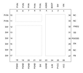
Figure 4. Pin Assignment (Bottom View)
