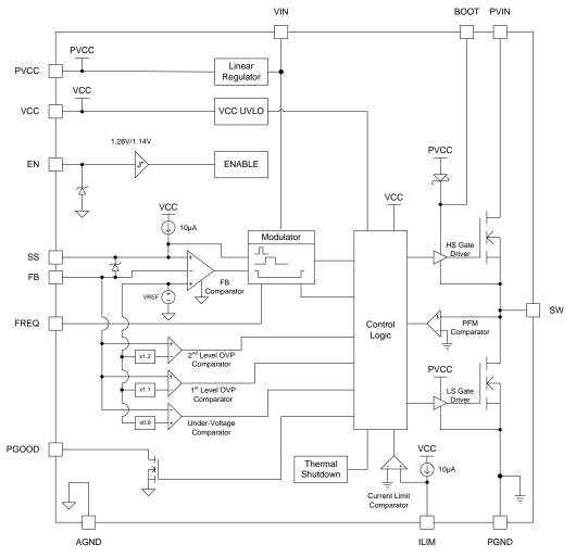
Figure 3. Block Diagram
