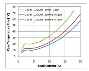
Figure 12. Case Temperature Rise vs. Load Current on Figure 13. Case Temperature Rise vs. Load Current 4 Layer PCB, 1 oz Copper, 7 cm x 7 cm on 4 Layer PCB, 1 oz Copper, 7 cm x 7 cm
