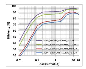
Figure 6. Efficiency vs. Load Current with  $V_{\text{IN}}$ =19 V and  $f_{\text{SW}}$ =500 kHz
