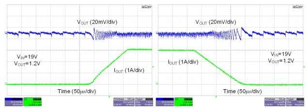
Figure 22. Operation as Load Changes from 0 A to 3 A Figure 23. Operation as Load Changes from 3 A to 0 A
