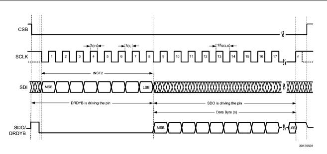
FIGURE 24. Timing Protocol for DrdybCase1
