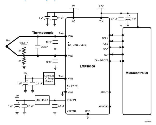
FIGURE 40. Thermocouple with CJC
