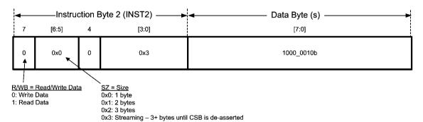
FIGURE 36. Setting up SPI\_STREAMCN
