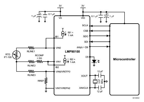
FIGURE 38. Topology #1: 3-wire RTD Using 2 Current Sources
