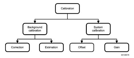
FIGURE 12. Types of Calibration
