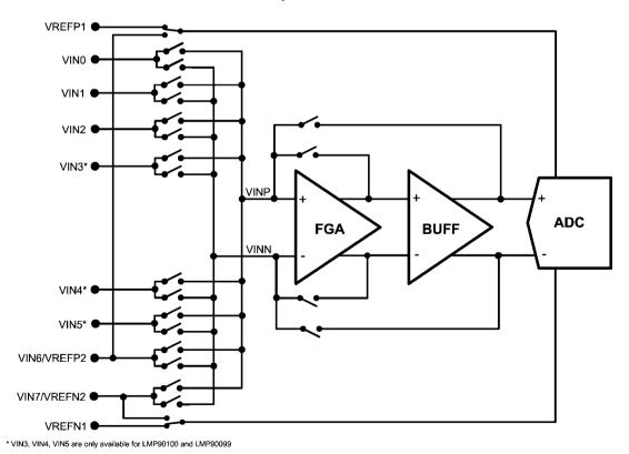
FIGURE 3. Simplified VIN Circuitry
