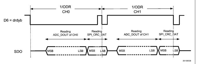
FIGURE 29. Timing Protocol for Reading SPI\_CRC\_DAT beyond normal DRDYB deassertion at every 1/ODR seconds
