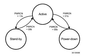
FIGURE 30. Active, Power-Down, Stand-by State Diagram
