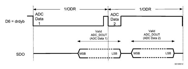
FIGURE 22. DRDYB Behavior for an Incomplete ADC\_DOUT Reading
