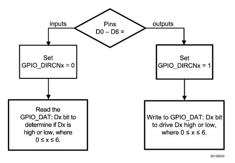
FIGURE 11. GPIO Register Settings
