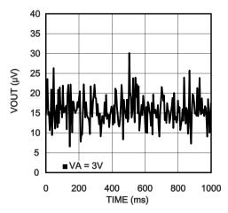
Noise Measurement with Calibration at Gain = 8
