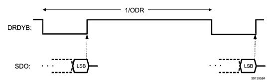
FIGURE 20. DRDYB Behavior for a Complete ADC\_DOUT Reading
