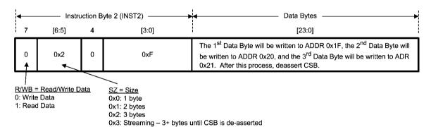
FIGURE 32. Register-Write Example 1
