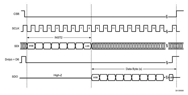
FIGURE 27. Timing Protocol for DrdybCase3
