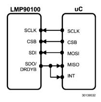
FIGURE 23. DrdybCase1 Connection Diagram
