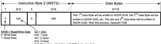
0x3: Streaming – 3+ bytes until CSB is de-asserted
