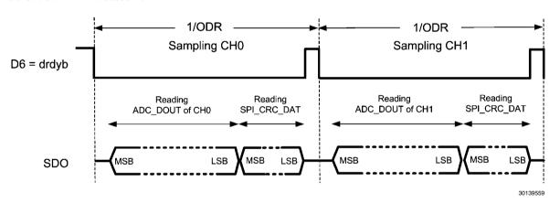
FIGURE 28. Timing Protocol for Reading SPI\_CRC\_DAT
