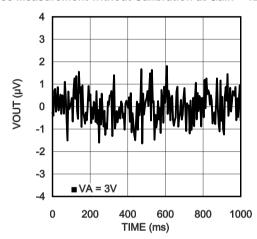
Noise Measurement without Calibration at Gain = 128
