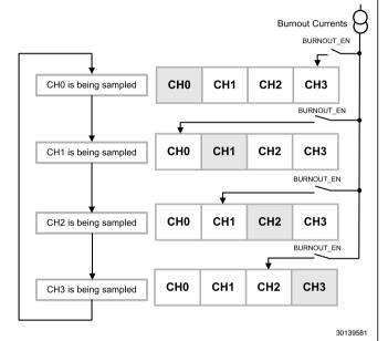
FIGURE 17. Burnout Currents Injection for ScanMode3
