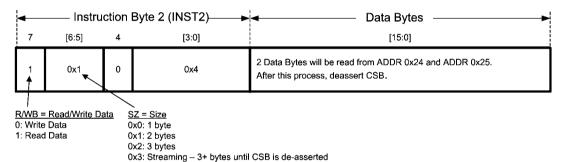
FIGURE 34. Register-Read Example
