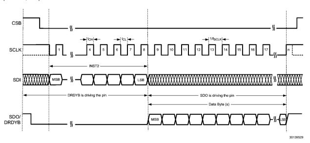
FIGURE 25. Timing Protocol for DrdybCase2
