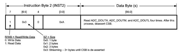
FIGURE 37. Controlled Streaming Example
