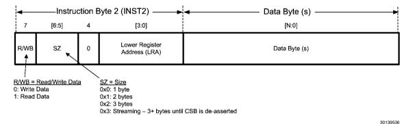
FIGURE 19. Register Read/Write Protocol
