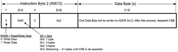
FIGURE 33. Register-Write Example 2
