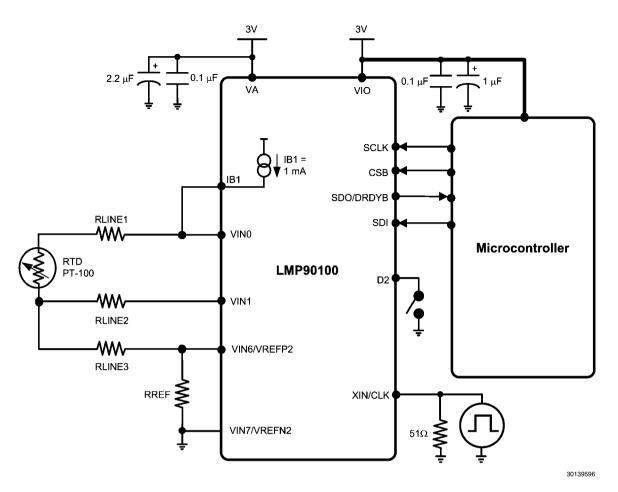
FIGURE 39. Topology #2: 3-wire RTD Using 1 Current Source
