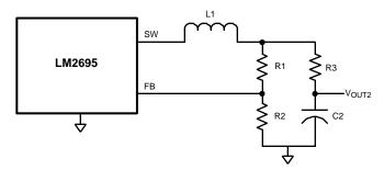
Figure 5. Low Ripple Output Configuration
