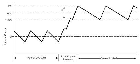
Figure 8. Inductor Current - Current Limit Operation
