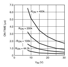
Figure 4. ON-Time vs V<sub>IN</sub> and R<sub>ON</sub>
